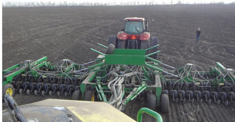
Figure 4.3. Semoir pneumatique John Deere (Commodity Air Cart 1910 + No-III Air Drill 1890).
