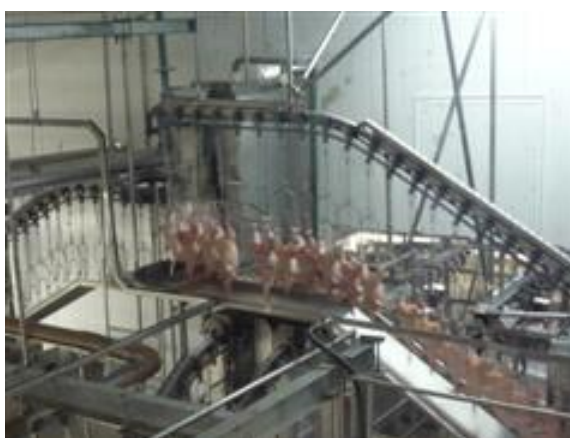
Figure 3 – End of first stage: after hanging, stunning, bleeding and plucking, the birds pass through the federal inspection and move on to next step
