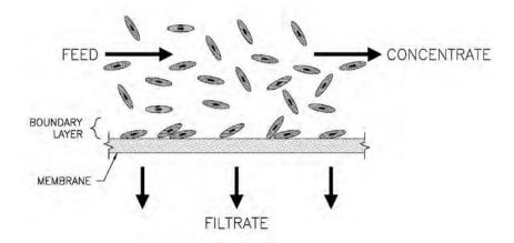
Figure 1.10: Principle of suspension mode filtration (USEPA, 2005).
