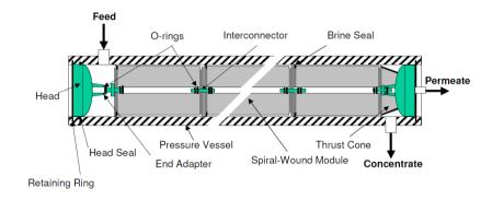
Figure 1.4: Typical spiral-wound module pressure vessel (from (USEPA, 2005)).
