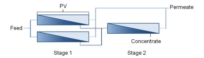
Figure 1.3: Simplified schematic of an RO train.
