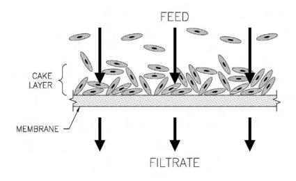
Figure 1.9: Principle of deposition mode filtration (USEPA, 2005).
