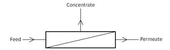
Figure 1.1: Schematic representation of the RO membrane process.
