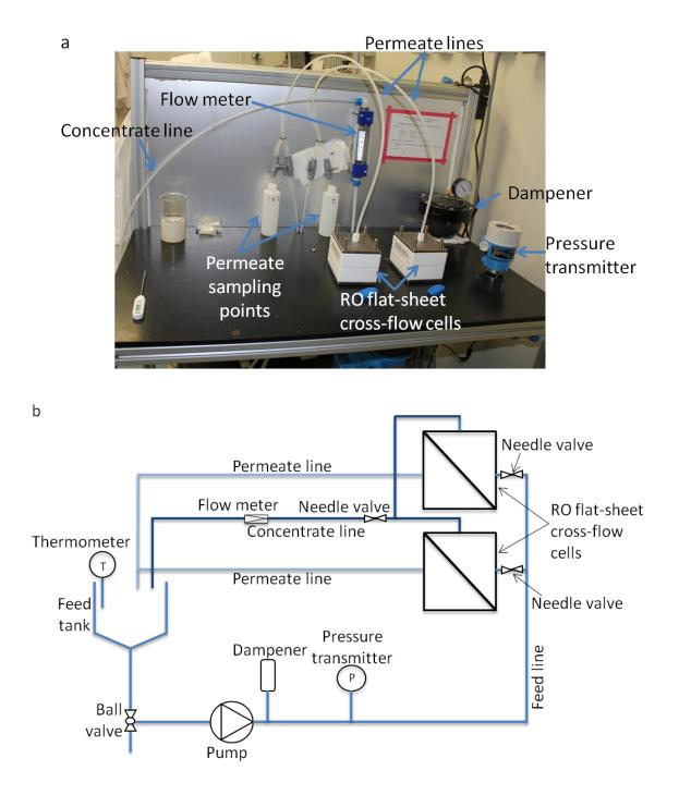
Figure 2.3: (a) photo and (b) drawing of the plastic flat-sheet set-up.
