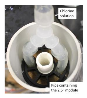
Figure 5.5: Picture of the 2.5" spiral-wound module ageing set-up.
