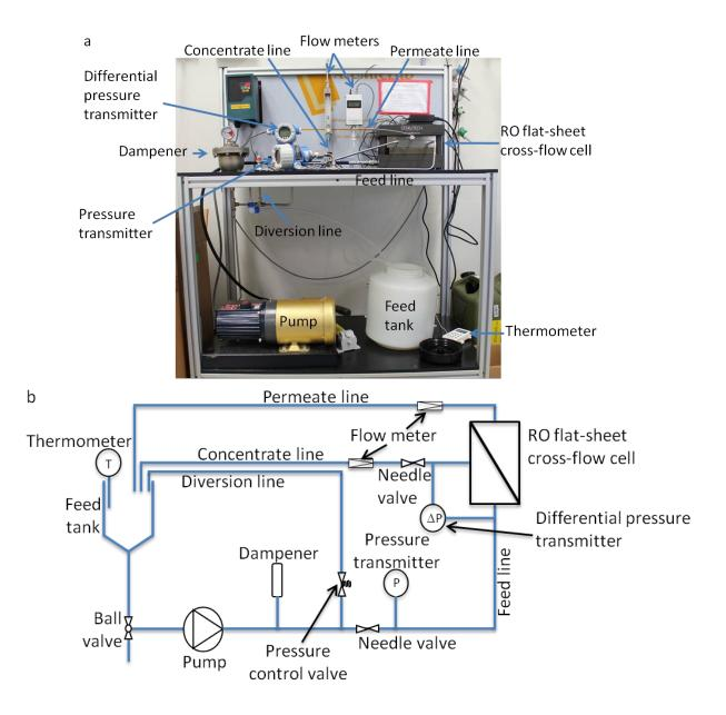
Figure 2.2: (a) photo and (b) drawing of the SS flat-sheet set-up.
