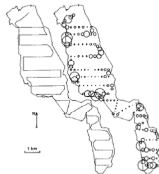
Figure 1. Echo-integration results of Lake Annecy. Left: location of hydroacoustics transects. Right: plots of echo-integration values, for two minute sequences. Each circle is proportional to the echo-integration units for the layer 0-25 m.
