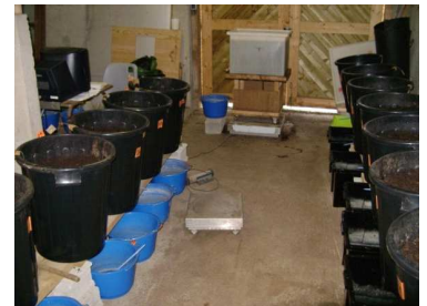
Figure 27. Large scale vermifilter and not insulated building for mesocosm experiment; both received the same liquid added each day
