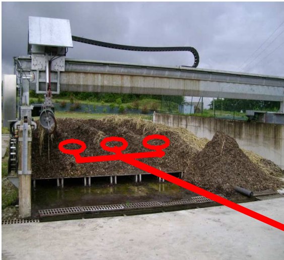
Figure 27. Large scale vermifilter and not insulated building for mesocosm experiment; both received the same liquid added each day
