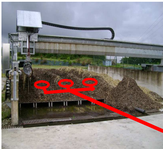
Figure 14. Large scale vermifilter and mesocosm experiment in a not insulated building; both received the same liquid added each day
