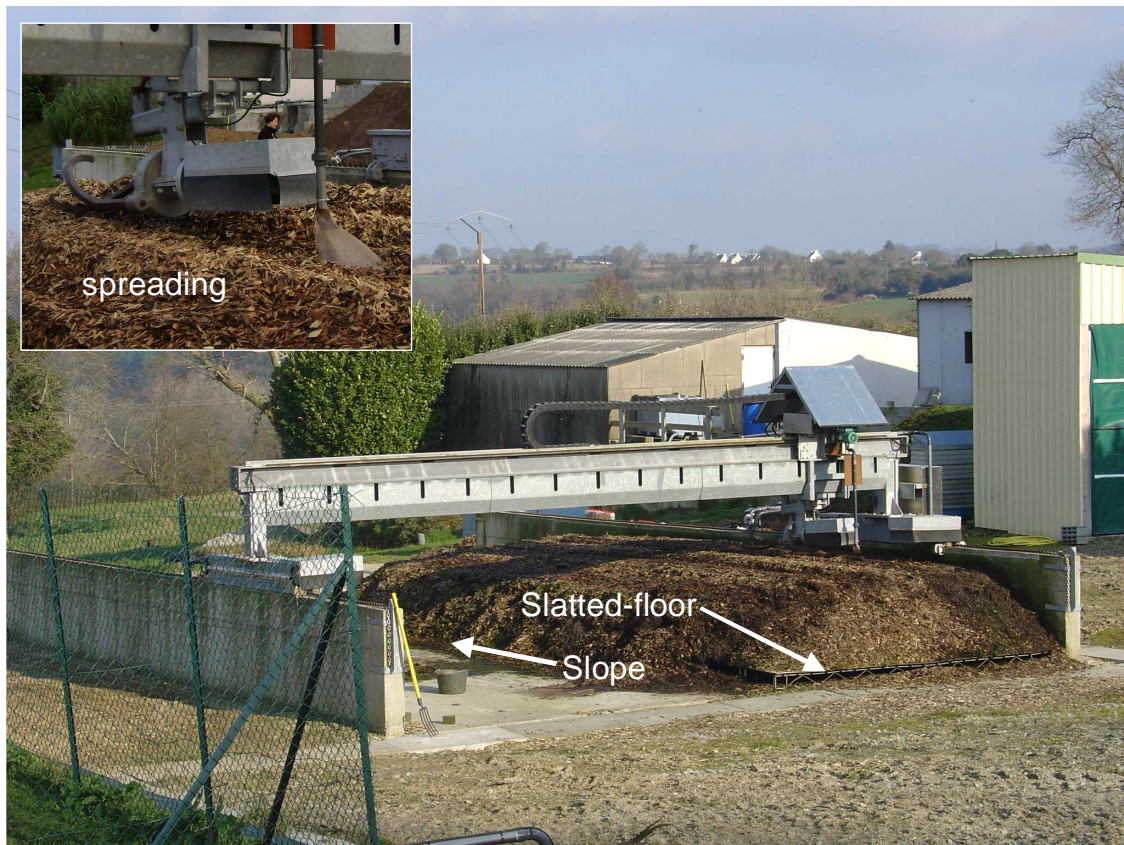
Figure 10. Vermifilter (width: 4m, length: 10m, height: 0,6m)
