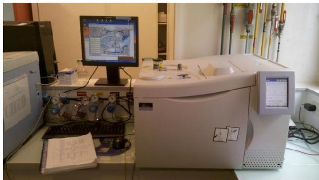
Figure I-9 : Chromatographe Clarus 580 (Perkin Elmer)
