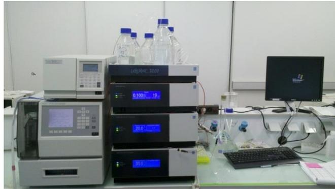
Figure I-8 : Chromatographe liquide haute performance (HPLC)
