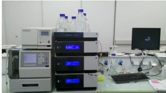
Figure I-8 : Chromatographe liquide haute performance (HPLC)
