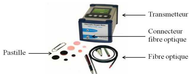
Figure 57 : Sonde PreSens Fibox PSt 3
