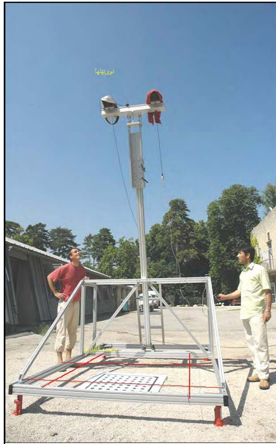
Figure 2: Support and camera system used for stereoscopic vision.
