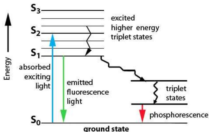
Figure 1 : Jablonski diagram of excitation and emission of a molecule in fluorescence or phosphorescence (Lakowicz, 1983)
