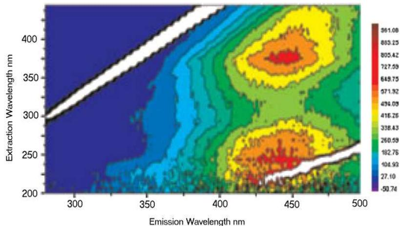
Figure 2 : Typical Excitation Emission Matrix (EEM) in a water sample (Hudson et al., 2007)
