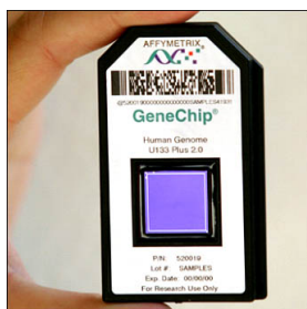
Figure 1.25: Affymetrix GeneChip ® used to quantify mRNA expression.
