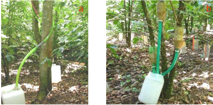
Photography 6. Detailed views of measurements of Inga stemflow (a) and coffee stemflow (b) on the research station of CICAPE, San Pedro de Barva, Heredia, Costa Rica.
