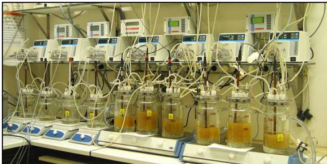
Figure 2.3: Simulator of the human intestinal microbial ecosystem (SHIME model).
