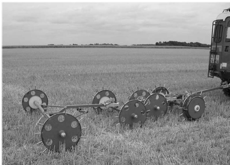
**Figure II-3:** MUCEP “Multi Continuous Electrical Profiling”.
