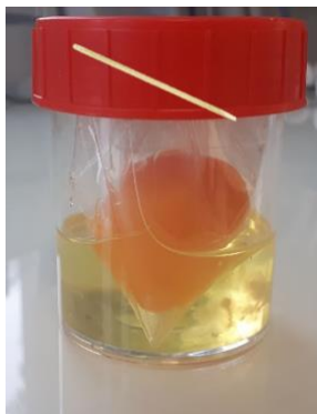
Figure 2.3. Picture of the dialysis bag egg model placed in a 125 mL sterile vessel. The homogenised EW was inoculated with 10^7 CFU/mL washed cells. The sterile yolk was confined in a dialysis bag sealed with a toothpick (12-14 kDa; 4.8 cm diameter) and immersed in EW. The vessel was hermetically closed and incubated at 30 °C.
