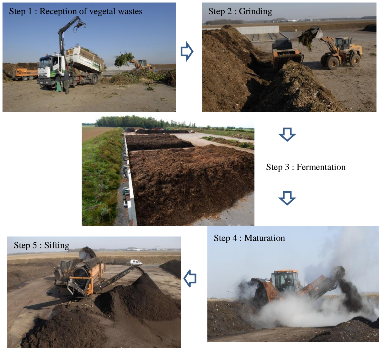
Fig. 6- 5. Processes to make green waste compost. Source: the website of a green waste compost platform called “Ferme de La Martinière” in Saclay of Ile-de-France.
