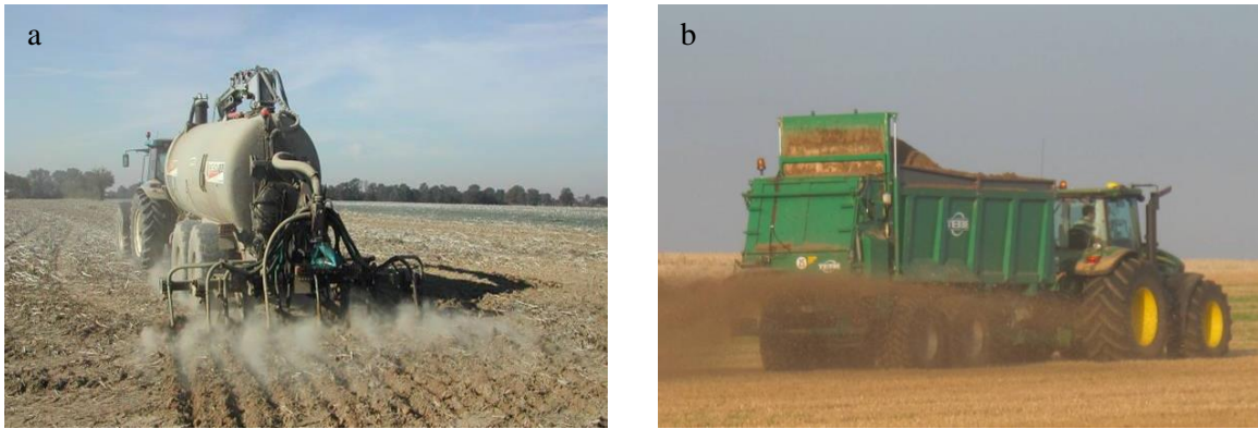
Fig. 6-3. Agricultural land application of sewage sludge. a. liquid sludge, b. solid sludge. Source: the site of Valterra, an enterprise specialized in agricultural reclamation of urban waste
