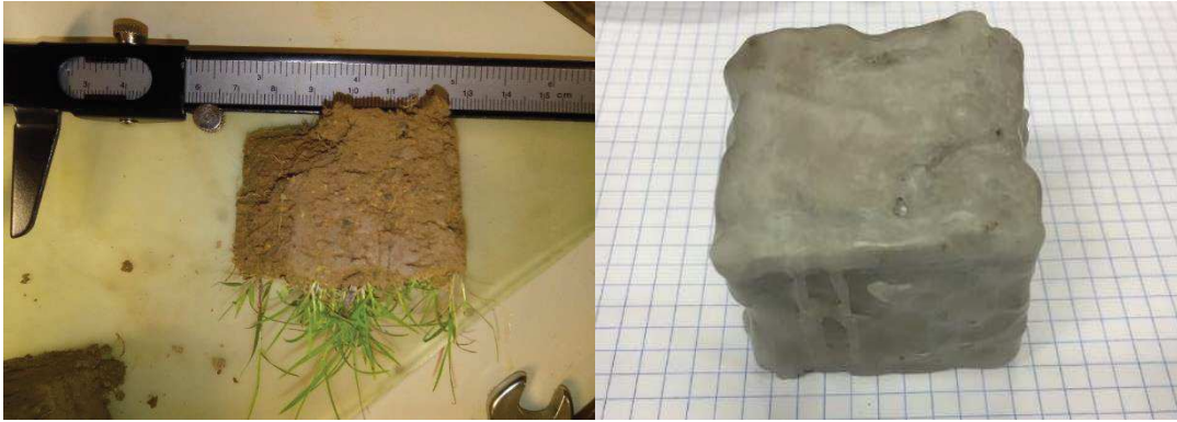
Figure 11 Paraffin tests on vegetated soil: a) before and b) after soil covering
