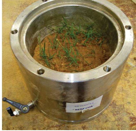
Figure 20 Large size oedometer cell, with vegetated sample inside.
