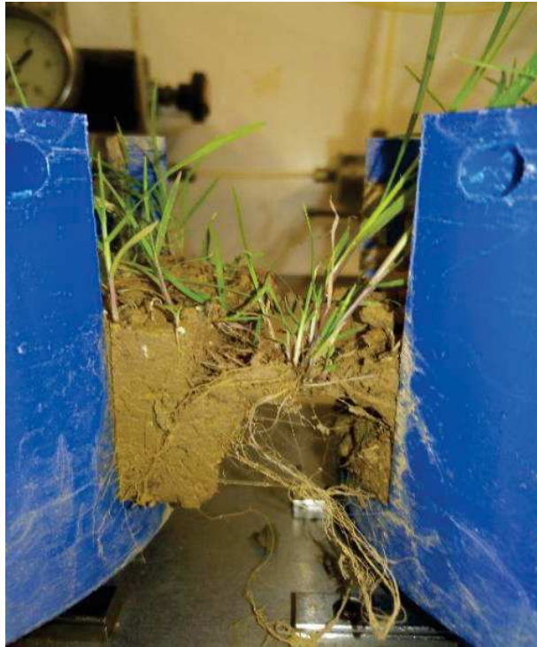
Figure 46 Unbroken roots after test, within the fissure generated by the tensile test
