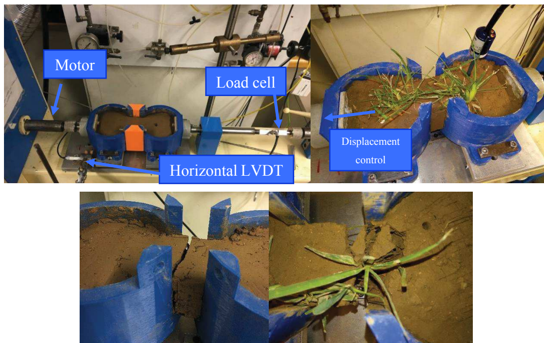
Figure 39 Tensile test equipment in its initial configuration, before testing. A) On the left-hand-side: the motor for controlled displacement and the horizontal LVDT. On the right-hand-side: the load cell. B) Bridge supports removed, and direction of the traction displacement imposed by the motor. C) End of test and fissure generated in bare soil D) End of test and fissure generated by tensile displacement in vegetated soil. Roots visible within the fissure.
