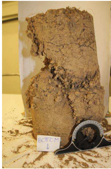
Figure 42 Stress strain behaviour under triaxial compression of bare and vegetated soils at a) low suction, low confinement b) high suction, high confinement stress. The respective volumetric deformations are in c and d. E) samples in which brittle behaviour was observed, with a peak in the deviatoric stress and f) respective volumetric behaviour. G) shear band observed during visual inspection of a vegetated sample after triaxial compression
