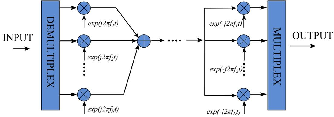
Figure 4.1 — Block diagram of a generic FDM system
