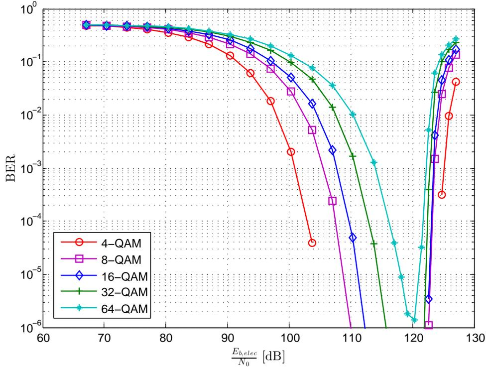
Figure 4.8 — BER performance of DCO-OFDM versus electrical SNR at the transmitter for different modulation orders,  $\kappa = 10$  dB and  $R_b/f_c = 10$  in this case.
