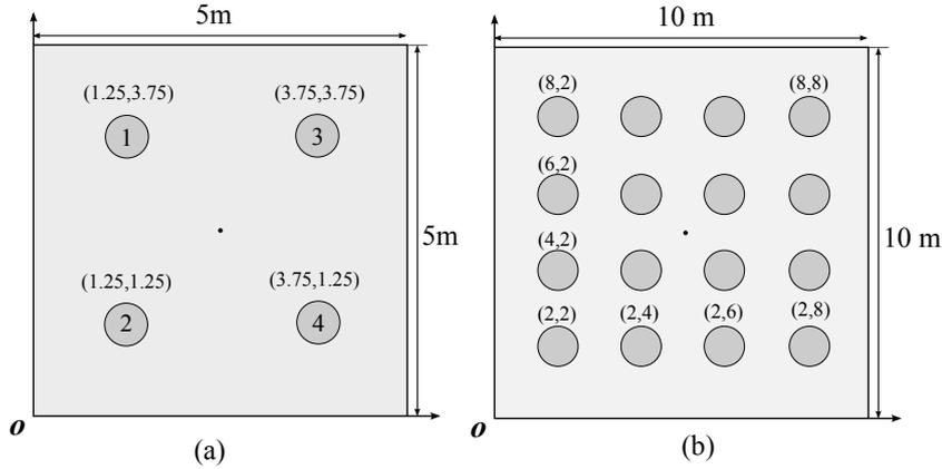
**Figure 3.4** — The layout of LEDs on the ceiling for the two cases of: medium-size (a), and large (b) rooms of dimensions  $(5 \times 5 \times 3) \text{ m}^3$  and  $(10 \times 10 \times 4) \text{ m}^3$ , respectively.
