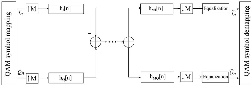
**Figure 5.2** — Block diagram of conventional CAP transceiver,  $M$  is the up-sampling factor,  $h_I[n]$  and  $h_Q[n]$  are the digital in-phase and quadrature shaping filters, and  $h_{MI}[n]$  and  $h_{MQ}[n]$  are the corresponding MFs
