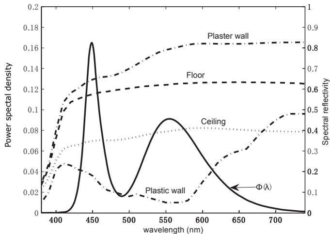
Figure 3.3 — Power spectral density  $\Phi(\lambda)$  of a white LED (solid line, which corresponds to the left axis) and the measure spectral reflectance (which corresponds to the right axis) of plastic and plaster wall, floor, and ceiling, reproduced from Figure 1 in [44].
