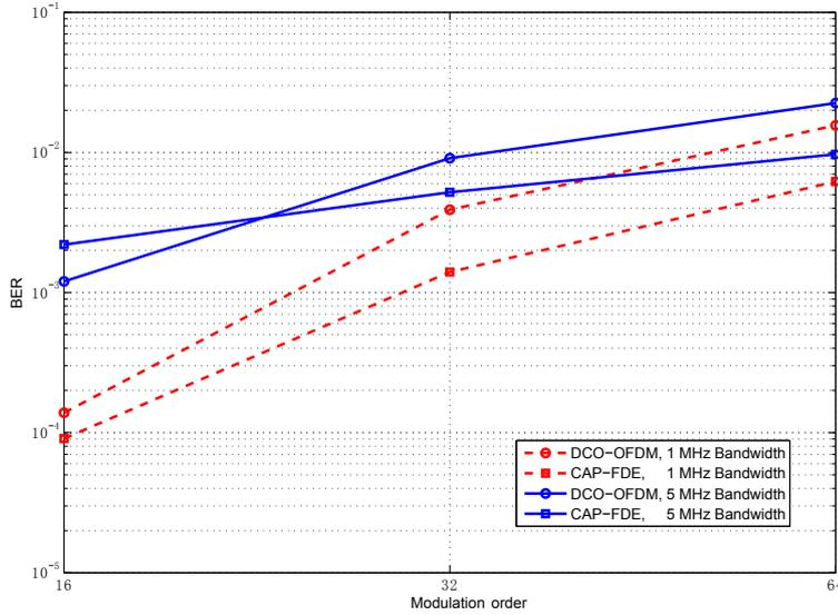
**Figure 7.6** — BER performance of DCO-OFDM and CAP-FDE (3V<sub>pp</sub>, 250mA DC bias) for different modulation order and signal bandwidth
