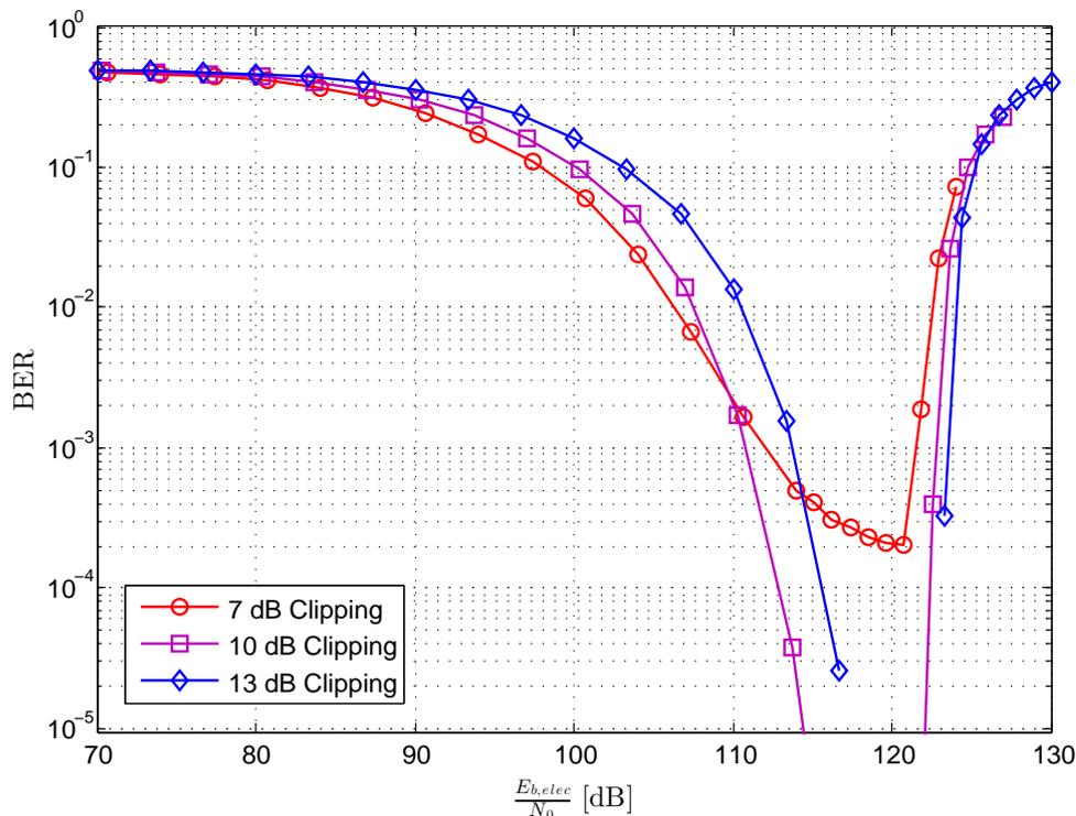
**Figure 4.9** — BER performance of 32-QAM DCO-OFDM versus electrical SNR at the transmitter for different clipping factors  $\kappa$ ,  $R_b/f_c = 10$ .
