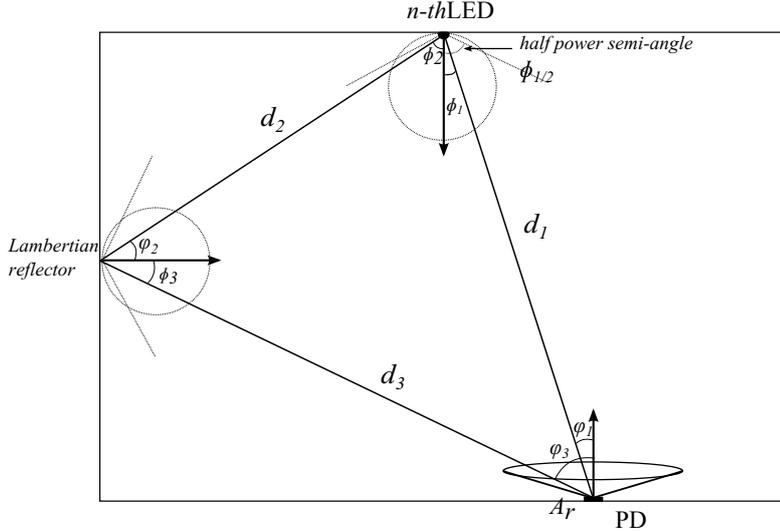
**Figure 3.1** — Propagation model for the indoor VLC channel.
