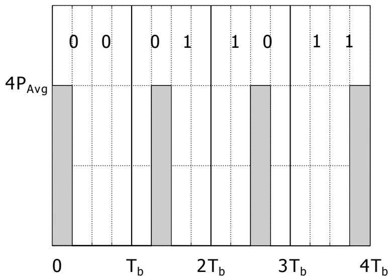
Figure 2.6 — An example of 4-PPM modulation
