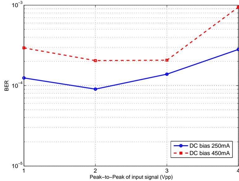
**Figure 7.7** — BER performance of DCO-OFDM (16-QAM, 1 MHz bandwidth) for different values of input signal power (in terms of  $V_{pp}$  at the AWG) and DC bias
