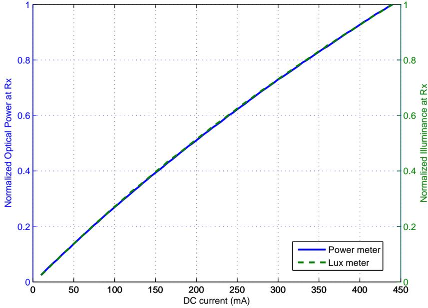
Figure 7.3 — Measured data of DC current versus output optical power and illuminance
