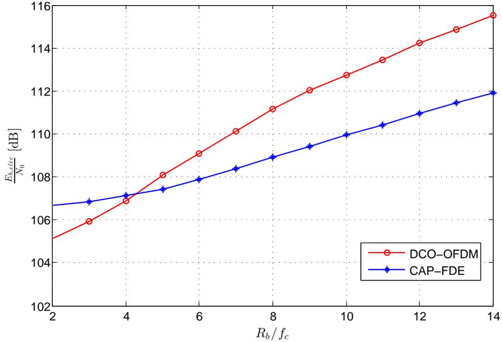
**Figure 5.9** — Electrical SNR at the transmitter versus  $R_b/f_c$  to achieve a BER of  $10^{-3}$  for 32-QAM DCO-OFDM and 32-CAP-FDE, the clipping factor is set to  $\kappa = 10$  dB
