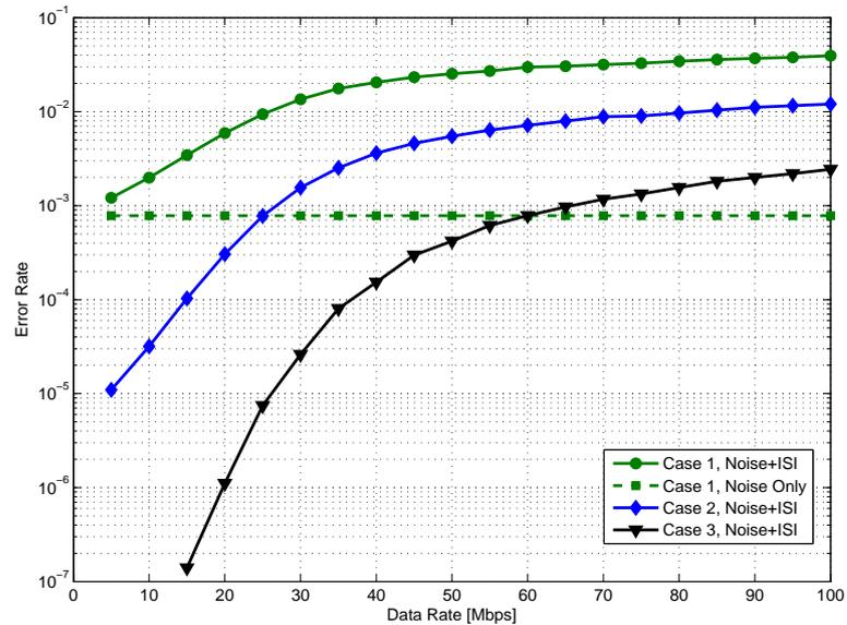
**Figure 3.8** — Receiver BER as a function of the data transmission rate for  $R_3$  position in the medium-size room. OOK modulation with MF at the receiver; Case 1:  $E_b/N_0 = 10$  dB, Case 2:  $E_b/N_0 = 13$  dB, Case 3:  $E_b/N_0 = 16$  dB.
