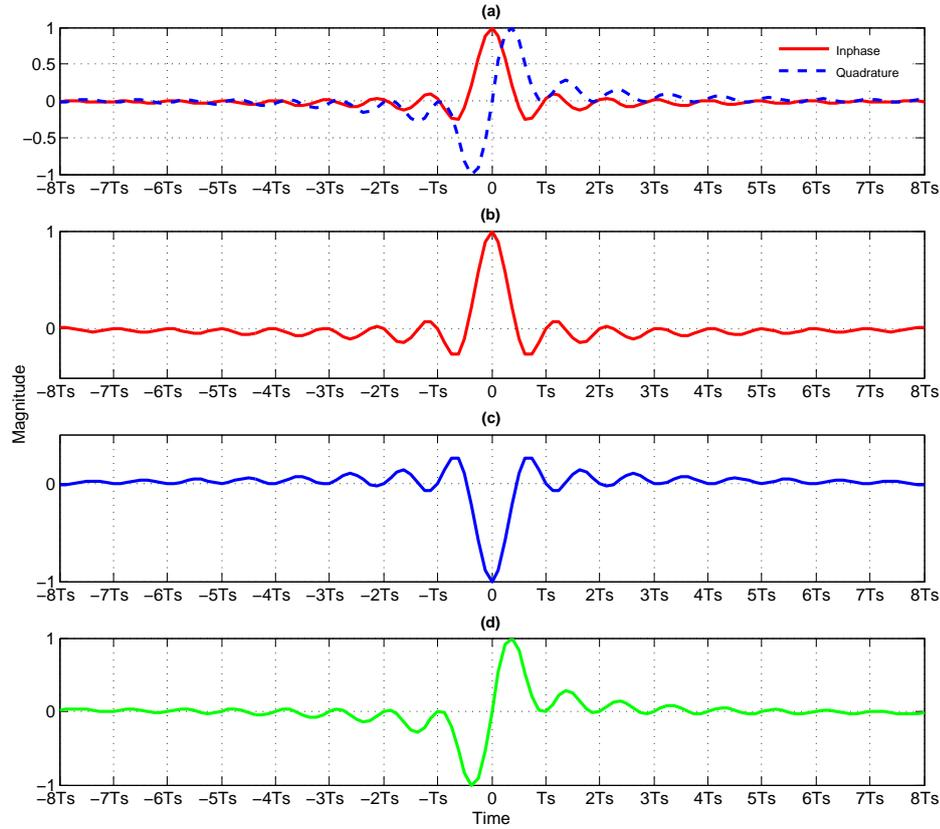
**Figure 5.3** — Impulse response of (a) Inphase and quadrature shaping filters (b)  $h_{II}(t)$  (c)  $h_{QQ}(t)$  (d)  $h_{IQ}(t)$ , RRCFs with  $\alpha = 0.1$
