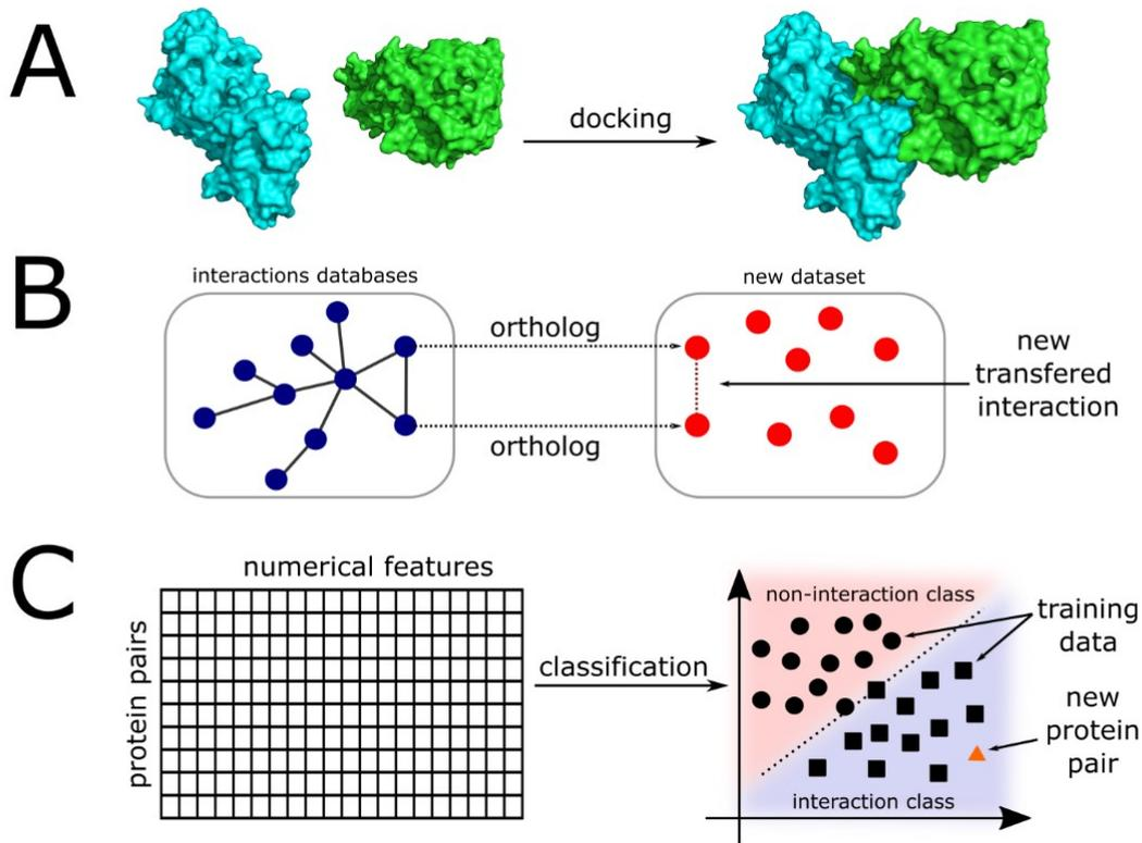
**Figure 9.** Examples of computational approaches for PPI prediction. A) Molecular docking, based on three-dimensional structures of potentially interacting pairs. B) Interolog methodology, based on interaction transfer for evolutionarily-related proteins. C) Machine learning approaches, which convert potentially interacting pairs in numerical representations for classification. Adapted from Keskin et al. (2016).
