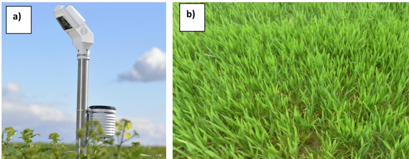
Fig. 2. a) The IoTA systems installed in a field. The top part inclined at  $45^\circ$  hosts the RGB camera. The cylinder attached to the vertical pole includes sensors to monitor the local air temperature and moisture. b) An example of a raw image.
