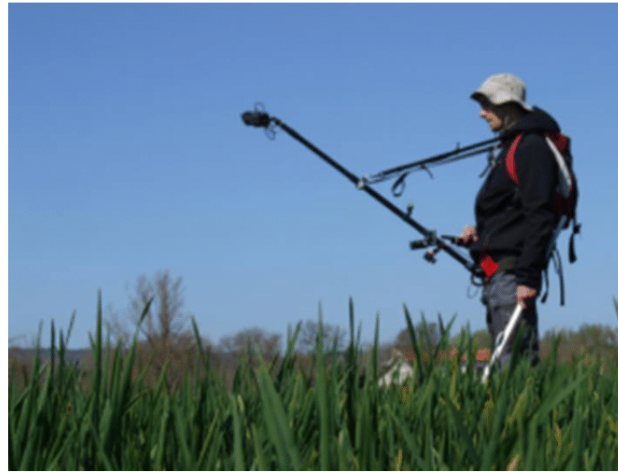
Figure 2 An operator acquiring images using the ground system consisting in a hand-held pole on the extremity of which the camera was fixed.
