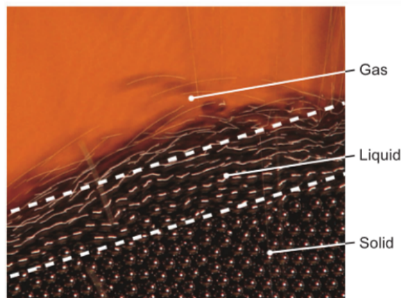
Figure 1.1 – The flow regimes of granular material : solid, liquid, gas obtained by pouring steel beads on a pile (Forterre and Pouliquen, 2008)
