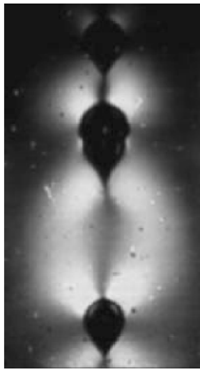
Fig. 2. Birefringence visualization: bubble volume V_B = 0.56 \times 10^{-6} \text{ m}^3/\text{s} ; injection period T = 0.2 \text{ s} ; 0.25% PAAm.
