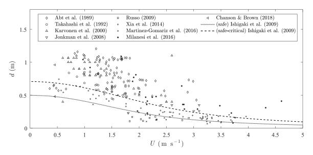
FIGURE 3.25. Human instability events in flood flows from different research works, and curves for safety evacuation during a flooding situation proposed by Ishigaki et al. (2009).
