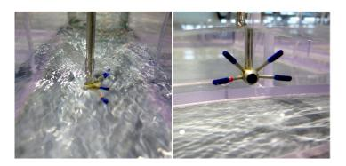
FIGURE 3.14. Acoustic Doppler Velocimeter (ADV) whit a sidelooking probe, fixed on the MURI mechanical gantry system.
