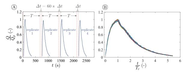
FIGURE 3.7. A) Inflow hydrograph replicates (only 4 of the 200 replicates are shown). The hydrographs do not cover fully the total duration, T, because the minimum discharge that the flowmeter is able to measure is  $0.13 \text{ ls}^{-1}$ . B) Overlapped inflow hydrograph replicates, using the starting point of the rising limb as a pivot point. In both plots, the discharges were normalized by the peak discharge,  $Q_p$ . The time t in plot B was normalised by the hydrograph rising time,  $T_r$ .
