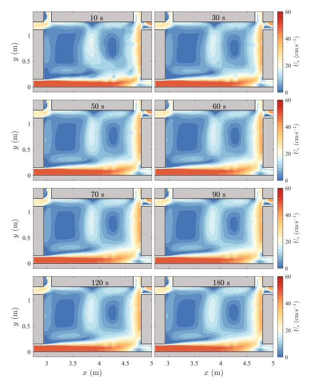
FIGURE A.2. Time-averaged surface velocity magnitude,  $U_s$ , for a town square configuration (without the city block), for increasing averaging durations, from 10 to 180 s.
