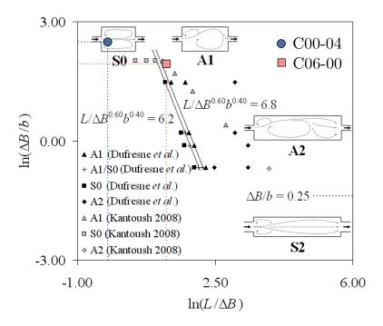
FIGURE 4.11. Classification diagram for flow patterns as a function of rectangular shallow reservoir geometry, from Dufresne et al. (2010). The points corresponding to the cases C00-004 (with an opening in the right and left walls of the block) and C06-00 (with an opening in the downstream and upstream walls) are indicated in the diagram.
