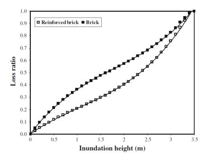
FIGURE 2.21. Loss ratio of reinforced brick and brick structures along with its contents at different flow depth for debris flows, from Lo et al. (2012).
