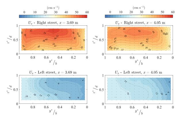
FIGURE E.2. Cross-sectional distribution of the time-averaged streamwise velocity in right and left streets corresponding to case C00-04 (Figure 4.1.C).
