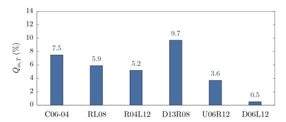
FIGURE 4.18. Discharge through the city block as a percentage of the total inflow discharge,  $Q_{in,T} = 6.5 \, \mathrm{l \, s^{-1}}$ , for the six flow cases corresponding to key issue 2.
