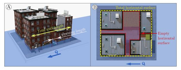
FIGURE 1.5. A) Isometric view of a city block, composed of four buildings. One opening is displayed in one side of the block. B) Plan view of a city block, showing the empty interior space in red color.
