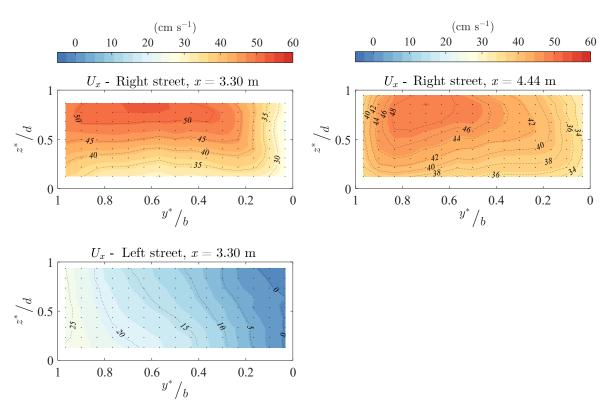
FIGURE E.1. Cross-sectional distribution of the time-averaged streamwise velocity in right and left streets corresponding to case C00-00 (Figure 4.1.A).
