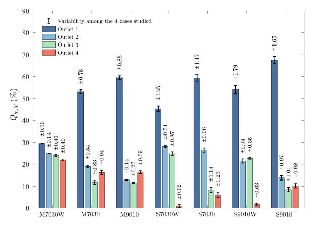
FIGURE 4.9. Discharge distribution at the different outlets for each set of experiments, values shown as a percentage of the total inlet discharge ( $Q_{in,T} = 6.5 \text{ ls}^{-1}$ ). The set of experiments M7030W corresponds to the original experiments.
