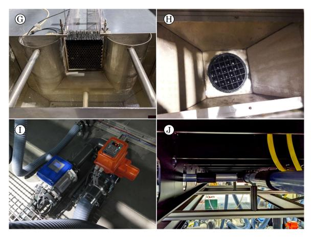
FIGURE 3.1. (Continued) G) Inlet tank, with a plastic honeycomb grid. H) Plastic grid in the connection between the inlet duct and inlet tank. I) Electromagnetic flowmeter (left) and an electrovalve (right), controlling the inflow discharge at each street. J) Pipes underneath the streets platform, which represents a sewer network.
