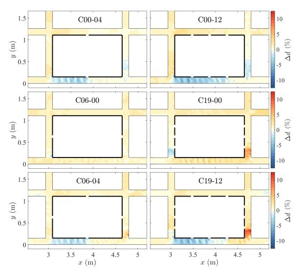
FIGURE 4.4. Relative difference in flow depth,  $\Delta d$  (Eq. 4.2), in the streets, with respect to the reference case C00-00, for cases corresponding to key issue 1. Warm colors indicate areas where flow depths are greater than in the reference case, while cool colours indicate areas where flow depths are smaller.
