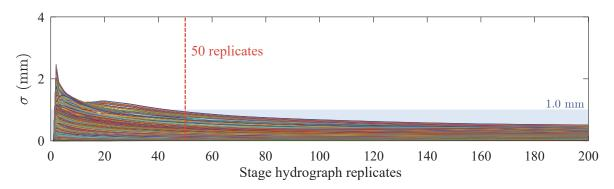
FIGURE 3.13. Ensemble-averaged standard deviation of the ensemble-averaged flow depths constituting the stage hydrograph at measuring point  $P_{in}$ . Convergence is reached when  $\langle \sigma \rangle_j(t) \leq 1$  mm (Eq. 3.6). This limit is indicated by the shaded area.
