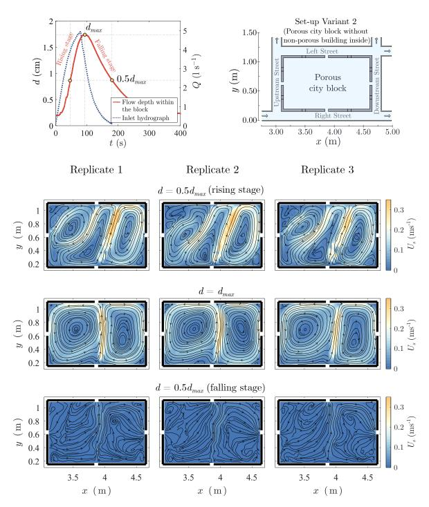
FIGURE 3.21. Average time-varying surface velocity, within the city block, for 3 replicates of the inflow hydrograph. The velocities are shown for the rising and falling stage, as well as at dmax. At the top, the inflow hydrograph is shown (blue dashed line), as well as the stage hydrograph measured within the block (red line), and the instant corresponding to each velocity map is indicated (yellow markers).
