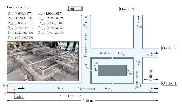
FIGURE 3.12. Schematics plan view of the experimental set-up variant 2, with the various locations of the measuring points of the flow depth, when addressing key issue 3. The schematic is not a scale, and the width of the streets has been distorted (enlarged) to fit all the required information.
