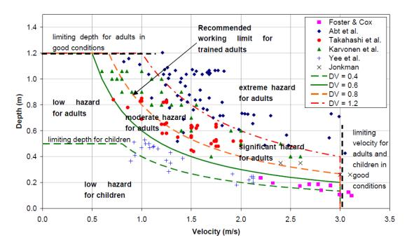
Figure 2.17. Flood hazard criterion for pedestrians proposed by Cox et al. (2010), with four levels of hazard. DV in the legend corresponds to Ud with present nomenclature.
