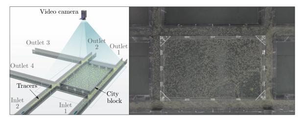
FIGURE 3.17. Left: Schematic of the set-up for the Large Scale Particle Image Velocimetry technique (LSPIV). Right: Plan view of the study area, showing the tracers on the flow surface during the implementation of the LSPIV technique.
