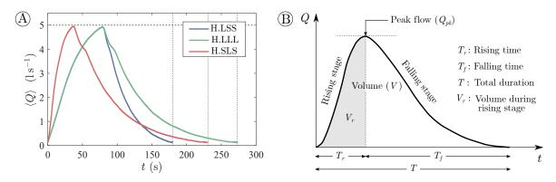
FIGURE 5.1. (A) Inflow hydrographs considered, listed in Table 5.1. The minimum recorded discharge is  $0.13 \ ls^{-1}$ , as explained in the Section 3.3.1.1. (B) Sketch of the inflow hydrograph characteristics listed in Table 5.1.
