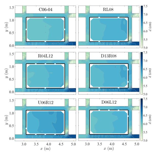
FIGURE 4.15. Flow depth (model scale), d, in the streets and within the city block for all flow cases corresponding to key issue 2. Deep blue colour indicates the greater flow depths and light colour indicates the shallower flow depths.
