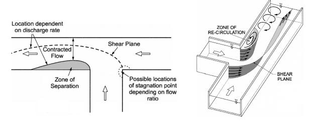
FIGURE 2.4. Flow characteristics in open-channel junction, from Weber et al. (2001).
