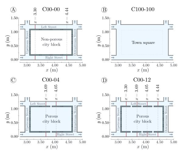
FIGURE 4.1. Top view schematics of the experimental cases corresponding to *key issue 1*. Red lines across the streets show the cross-section locations where discharges are estimated by the Velocity-Area method
