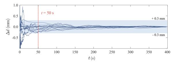
FIGURE 3.10. Convergence plot of the time-averaged flow depth at 13 various locations. Convergence is reached when  $\Delta$  (Eq. 3.4) is lower than the probe accuracy ( $\pm 0.3$  mm), showed by the shaded area.
