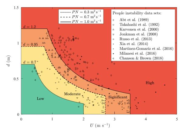
FIGURE 3.26. Proposed diagram for flood hazard to pedestrians, defining four levels of hazard. Based on available experimental data and field observations on people instability, and recommended guidelines for the safety of people during floods. Published in Mejía-Morales et al. (2021).
