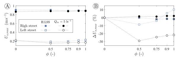
FIGURE 5.9. Maximum surface velocity,  $U_{s,max}$  and relative difference in maximum velocity,  $\Delta U_{s,max}$ , with respect to the reference scenario ( $\phi = 0$ ), as a function of the storage capacity of the city block, in right and left streets, for inflow hydrograph H.LSS and the steady flow case,  $Q_{in} = 5 \text{ ls}^{-1}$ .
