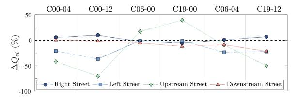
FIGURE 4.6. Relative difference in discharge with respect to the reference case,  $\Delta Q_{st}$ , at the upstream end of each street surrounding the urban block (i.e. at x = 3.09 m for the right and left streets and at y = 0.15 m for the upstream and downstream streets).
