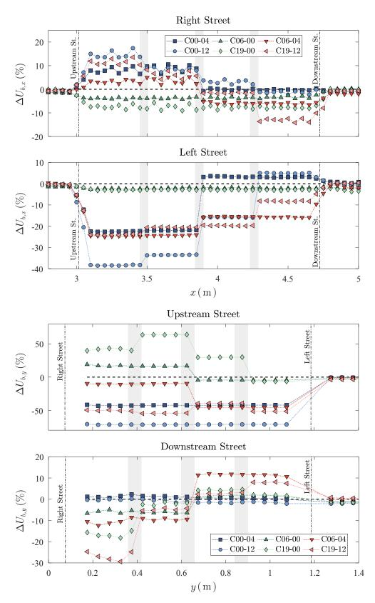
FIGURE 4.10. Relative difference in bulk velocity with respect to the reference case,  $\Delta U_{b,x}$  and  $\Delta U_{b,y}$ , in the longitudinal direction (x-axis) and transverse direction (y-axis), respectively. Vertical shaded bands indicate the location of the openings along the city block walls.
