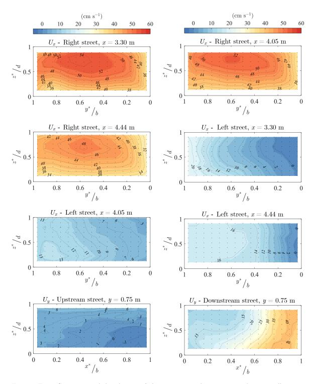
FIGURE E.8. Cross-sectional distribution of the time-averaged streamwise velocity in all streets corresponding to case RL08 (Figure 4.14.A).
