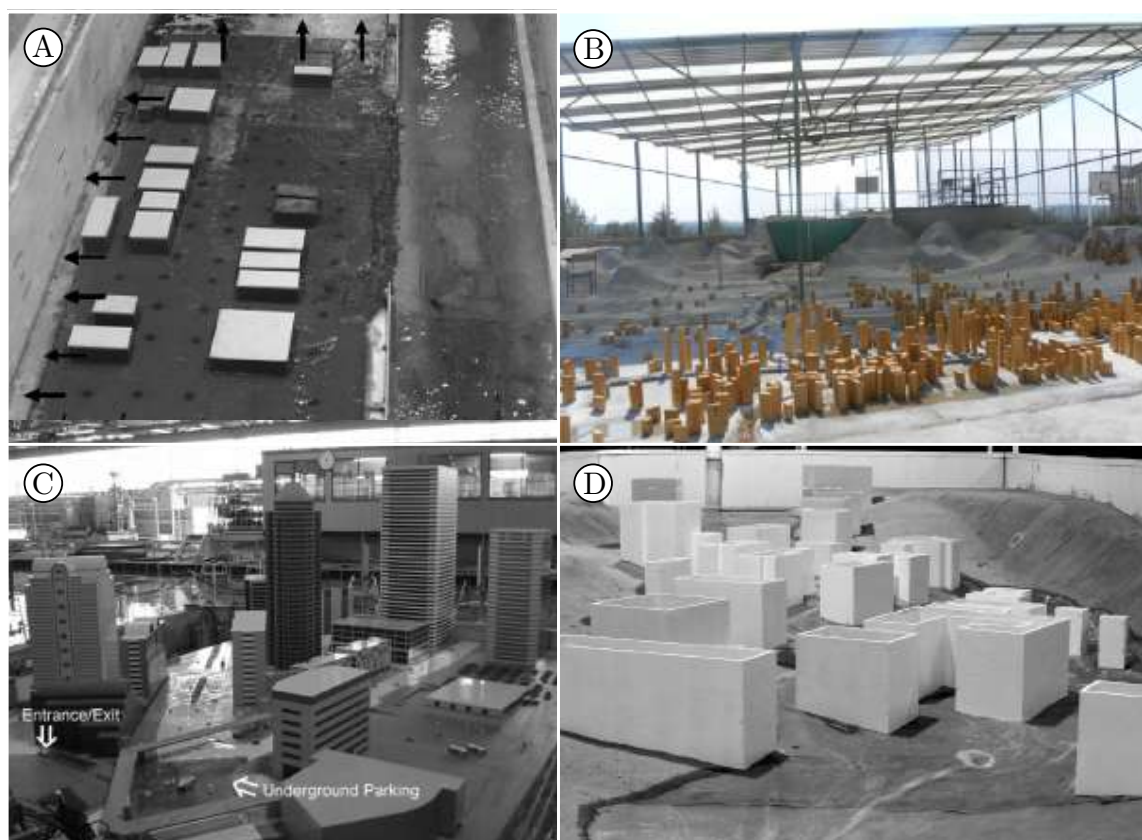
FIGURE 2.10. (A) Impervious plastic-coated wooden blocks, realistically aligned, for a fluvial flood experiment, from Sattar et al. (2008). (B) Realistic urban layout with impervious buildings, for dam-break-generated flood experiment, from Güney et al. (2014). (C) Realistic urban layout with impervious real-shaped buildings, for a coastal flood experiment, from Yasuda et al. (2004). (D) Realistic urban layout with impervious real-shaped buildings, for dam-break-generated flood experiment, from Smith et al. (2016).
