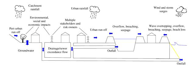
FIGURE 2.1. Integrated urban drainage, from Dawson et al. (2008).
