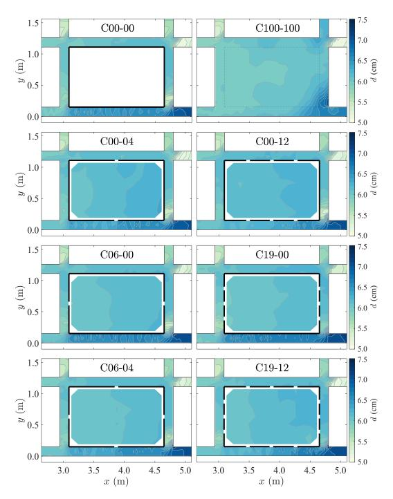
FIGURE 4.2. Flow depth, d (scale model), measured in the streets and within the city block for all flow cases corresponding to key issue 1. Deep blue indicates the greater flow depths and light colour indicates the shallower flow depths.
