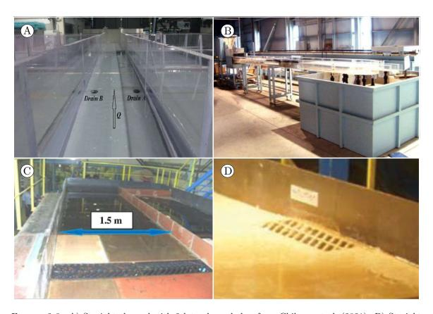
FIGURE 2.8. A) Straight channel with 2 lateral manholes, from Chibane et al. (2021). B) Straight channel with various central manholes, from Lee et al. (2012). C) Transverse grates, from Russo et al. (2013b). D) Rectangular grate, from Gómez et al. (2019).
