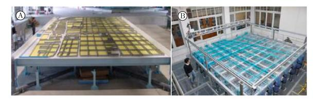
FIGURE 2.11. (A) Street network bounded by a real urban layout of impervious city blocks, for a fluvial flood simulation, from Ishigaki (2003). (B) Street network bounded by impervious city blocks in a synthetic urban area, for a fluvial flood simulation, from Finaud-Guyot et al. (2018).
