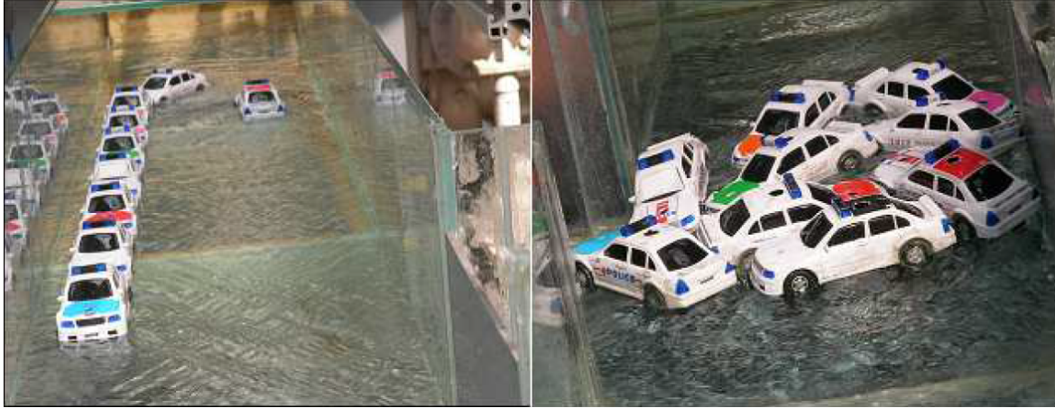
FIGURE 2.5. Leftt: Vehicles aligned with the direction of flow in the upstream branch. Right: Blockage of vehicles after being impacted by the flood wave., from Paquier (2009).
