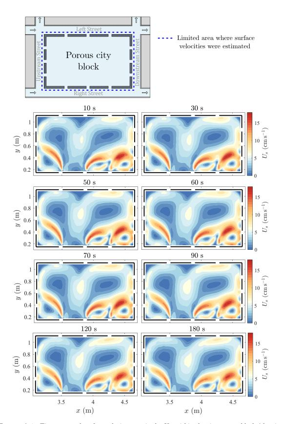
Figure A.1. Time-averaged surface velocity magnitude,  $U_s$ , within the city porous block (the city block has three openings in each wall), for increasing averaging durations, from 10 to 180 s.
