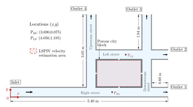
FIGURE 3.20. Location of the punctual areas in the streets and zone within the city block where the surface velocity was estimated by means of the LSPIV technique, for unsteady flow tests. The width of the streets is distorted (enlarged) in this schematic, to fit all the necessary information.
