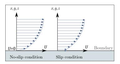
FIGURE 3.24. No-slip and slip boundary conditions. In no-slip noundary conditions, the flow velocity at the bundary is zero, whereas in slip boundary conditions there is relative movement between the boundary and the flow.
