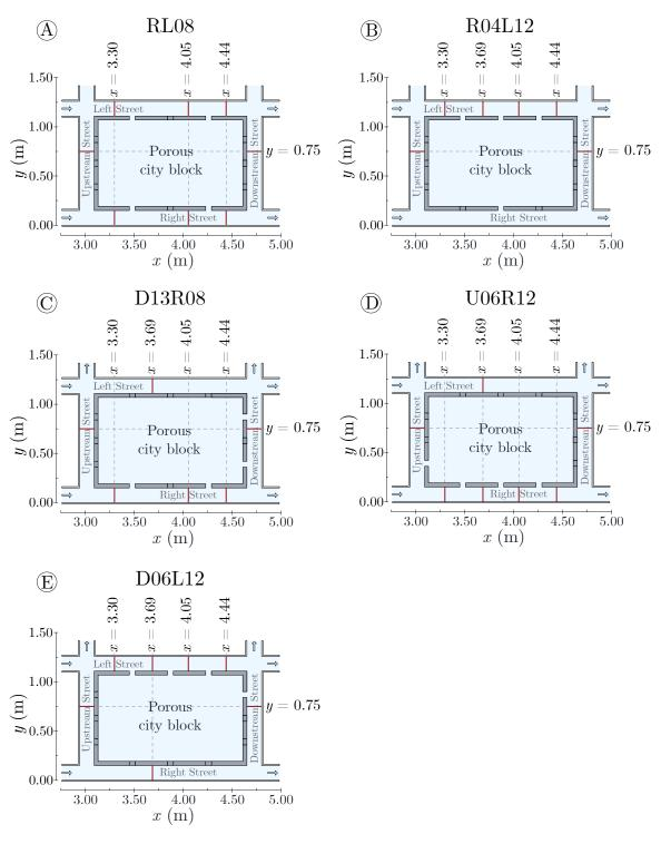
FIGURE 4.14. Top view sketches of the experimental cases corresponding to *key issue 2*, considered to study the conveyance porosity distribution. Red lines across the streets show the sections where ADV velocities are measured to compute the discharges by the Velocity-Area method.
