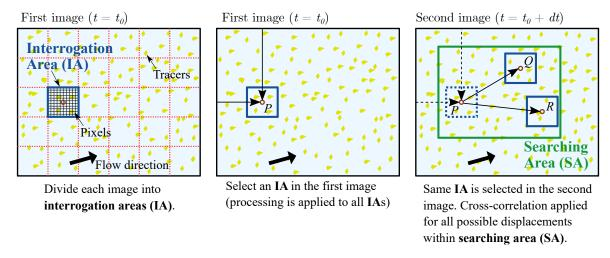
FIGURE 3.16. Conceptualization of the LSPIV image processing algorithm. Diagram replicated from Muste et al. (2008).
