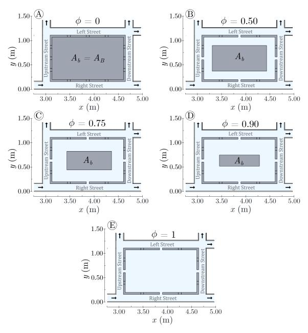
FIGURE 5.2. Variable block storage capacity,  $\phi$  (Eq. 5.4) within the city block. The case with  $\phi = 0$  serves as the reference flow condition.
