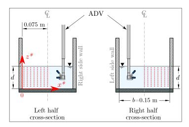
FIGURE 3.22. ADV velocity measurement grid in the street cross-section (red dots).  $x^*$  and  $z^*$  are local coordinates, which follow the direction of the global coordinates (x, y, z) and only change the position of the origin, in this case (street oriented along the y-axis) to the lower left corner of the street cross section.
