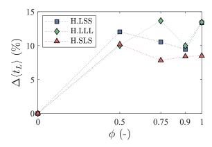
FIGURE 5.6. Relative change in time lag,  $\Delta \langle t_L \rangle$ , between the peak discharges of the inflow and global outflow hydrographs, with respect to the reference case ( $\phi = 0$ ) as a function of the storage capacity of the city block.
