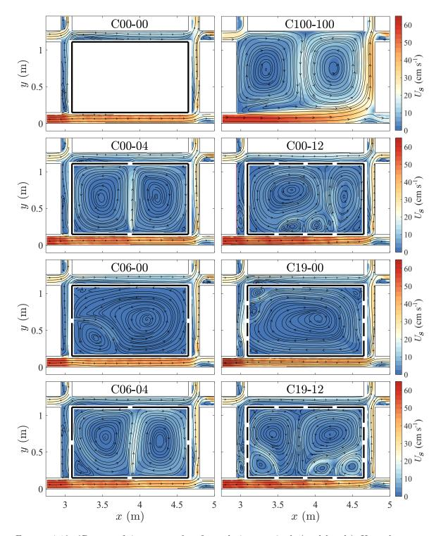
FIGURE 4.12. 2D maps of time-averaged surface velocity magnitude (model scale),  $U_s$ , and streamlines in the streets and within the city block (derived from LSPIV data), for all cases corresponding to  $key\ issue\ 1$ .
