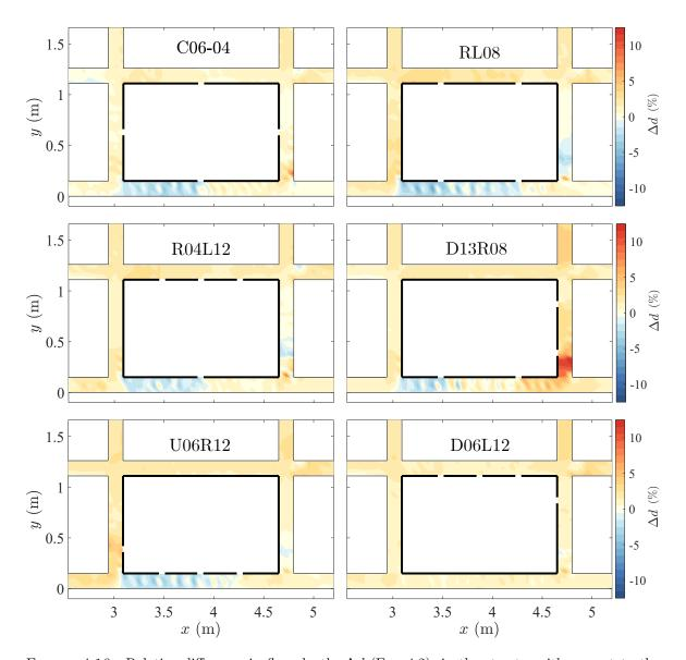
FIGURE 4.16. Relative difference in flow depth,  $\Delta d$  (Eq. 4.2), in the streets, with respect to the reference case C00-00 (from key issue 1), for cases corresponding to key issue 2. Warm colors indicate areas where flow depths are greater than in the reference case, while cool colours indicate areas where flow depths are smaller.
