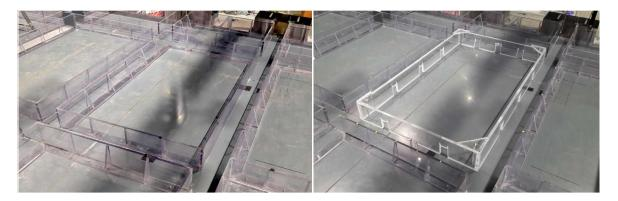
FIGURE 3.3. Left: Original non-porous city block. Right: Porous city block used in this PhD.
