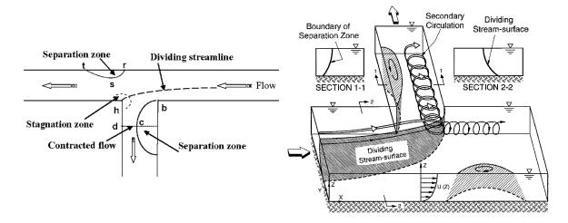
FIGURE 2.3. Flow characteristics in open-channel bifurcation. Scheme on the left taken from Ramamurthy et al. (2007), and on the right taken from Neary et al. (1999).
