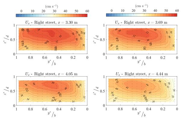
FIGURE E.7. Cross-sectional distribution of the time-averaged streamwise velocity in all streets corresponding to case C19-12 (Figure 4.1.H).
