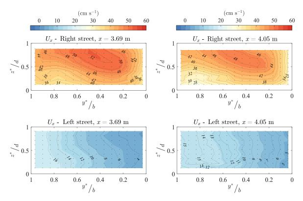
FIGURE E.6. Cross-sectional distribution of the time-averaged streamwise velocity in right and left streets corresponding to case C06-04 (Figure 4.1.G).
