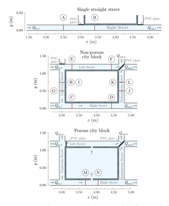
FIGURE B.2. Location of the cross-sections used for the evaluation of the different extrapolation scenarios.
