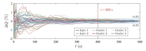
FIGURE 3.6. Time convergence of the time-averaged discharge for flowmeters located in the inlet and outlet conduits. Convergence is reached when  $\Delta Q \leq \pm 0.3 \%$  (Eq. 3.1). The shaded area indicates the convergence range ( $\pm 0.3 \%$ ).
