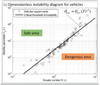
FIGURE 2.16. Sketch of the car geometry and definition of the mobility parameter. (a) definition of hazard criterion, (b) hazard criterion and (c) dimensionless instability diagram for flooded vehicles with identification of the critical threshold. Taken from Arrighi et al. (2016).
