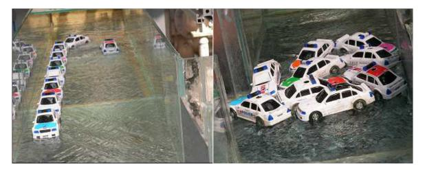
FIGURE 2.5. Left: Vehicles aligned with the direction of flow in the upstream branch. Right: Blockage of vehicles after being impacted by the flood wave., from Paquier (2009).
