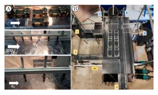
FIGURE 2.12. (A) Experimental set-up for a flow intrusion from a flooded street into a building under different conditions, from Mignot et al. (2020). (B) Experimental set-up with a synthetic building layout within a city block, from Li et al. (2021).
