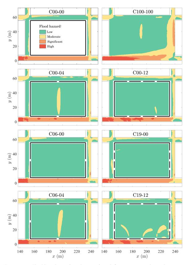
FIGURE 4.13. Flood hazard maps for pedestrians, for each flow case corresponding to *key issue 1*, obtained by scaling flow depths and velocities at the real-world prototype scale using Froude similitude (Eqs. 3.13 and 3.14).
