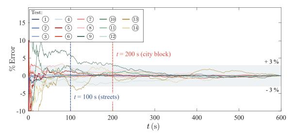
FIGURE 3.15. Time convergence of the time-averaged streamwise velocity (ADV) at 14 various locations. Convergence is reached when %Error  $\leq \pm 3\%$  (Eq. 3.7). The shaded area indicates the range  $\pm 3\%$ .
