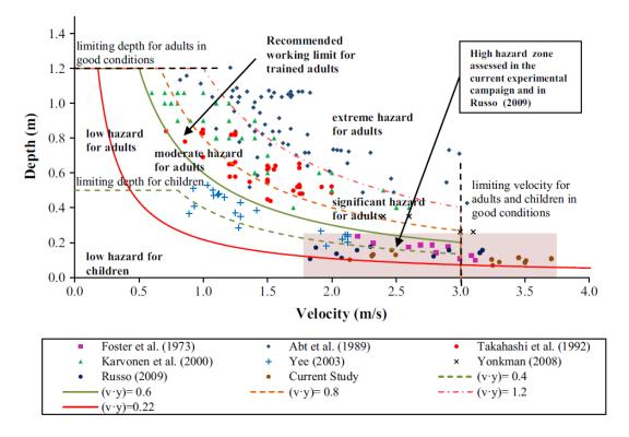
FIGURE 2.18. Human instability points and and threshold curve  $Ud = 0.22 \text{ m}^2 \text{ s}^{-1}$  from Russo et al. (2013a) and Martínez-Gomariz et al. (2016), integrated into the flood hazard criterion for pedestrians proposed by Cox et al. (2010). Taken from Martínez-Gomariz et al. (2016), where (v·y) in the legend corresponds to Ud in present nomenclature.
