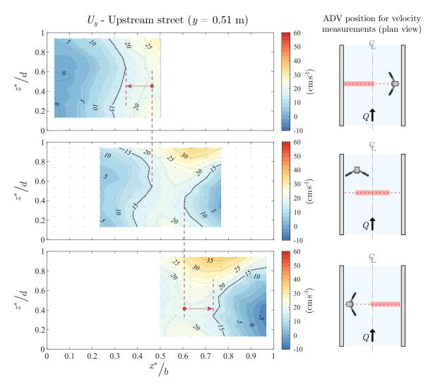
FIGURE C.2. Cross-sectional distributions of the time-averaged velocity in the upstream street. At the top, the left half section, measured with the ADV placed on the right side, in the middle the central section, measured with the ADV placed in front of the flow and at the bottom the right half section measured with the ADV placed on the left side of the street.
