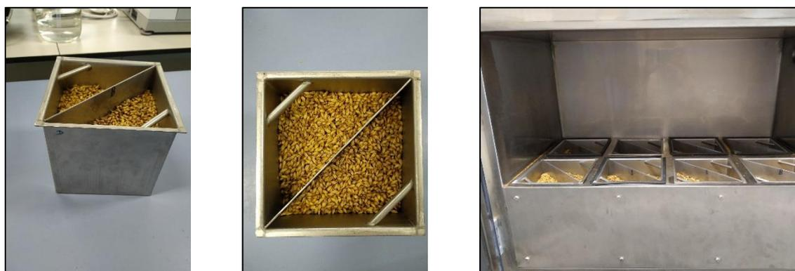
**Figure 5.1 Baskets for pilot-scale kilning experiments and micro-malting equipment**
