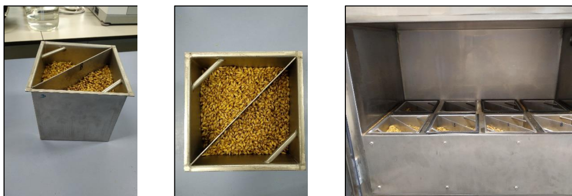
Figure 5.1 Baskets for pilot-scale kilning experiments and micro-malting equipment
