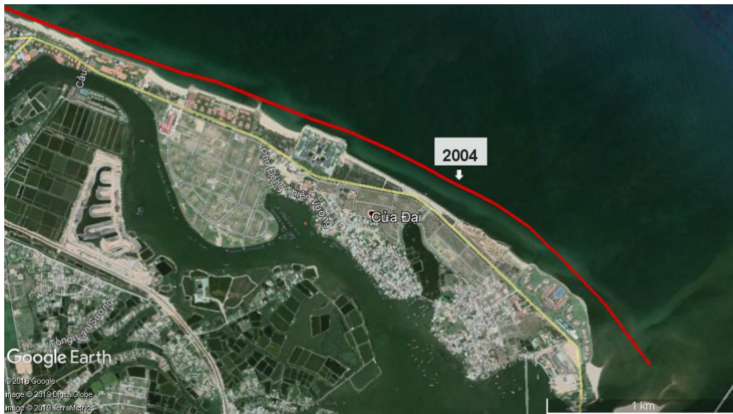
Figure 4.1: Coastal erosion in Hội An between 2004 and 2018
