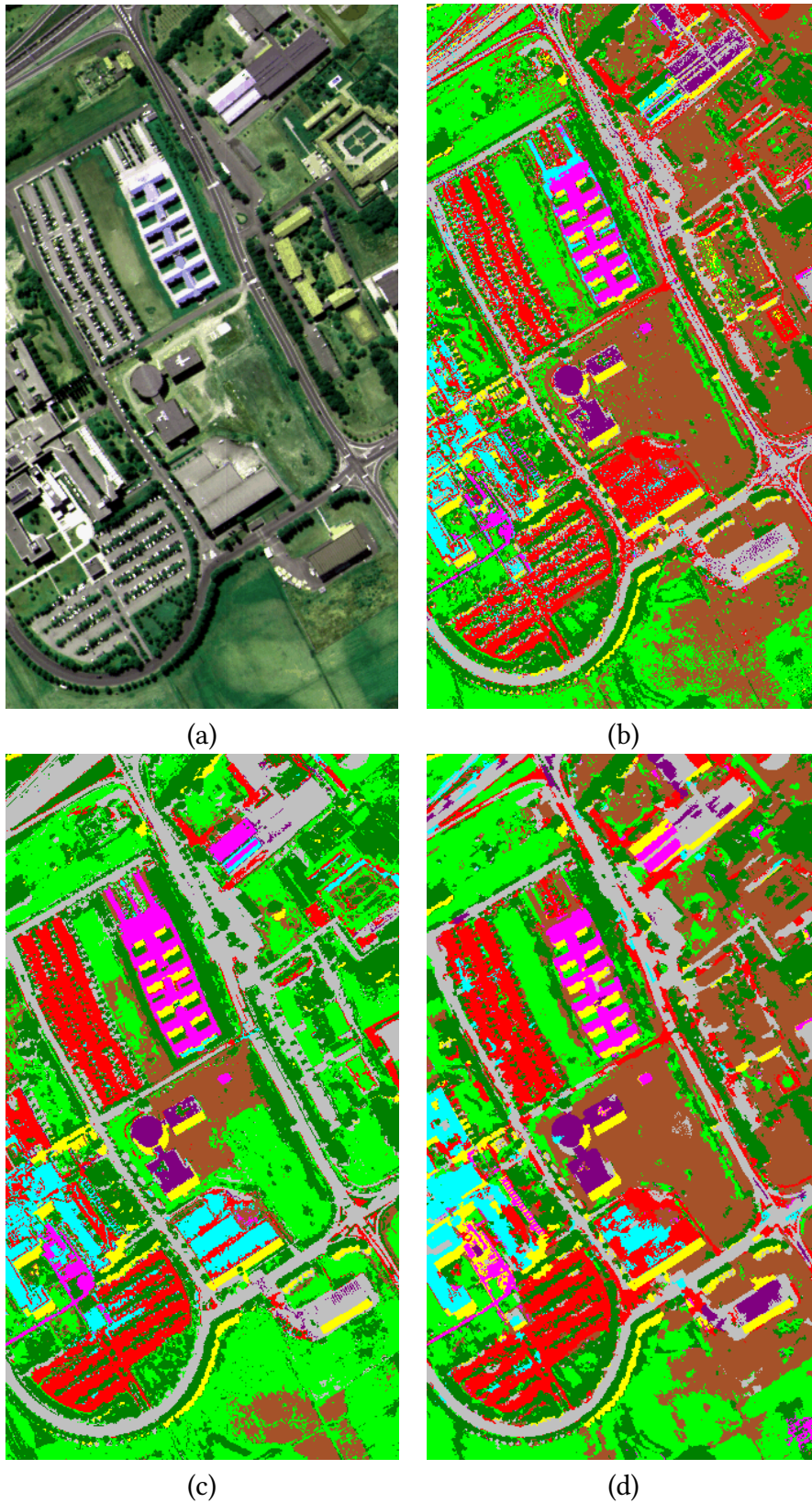
Figure 2.7.: (a) False color original image of University Area. (b) Classification map using the RBF kernel. (c) Classification map using the EMP. (d) Classification map using the proposed kernel where \lambda = 30 .
