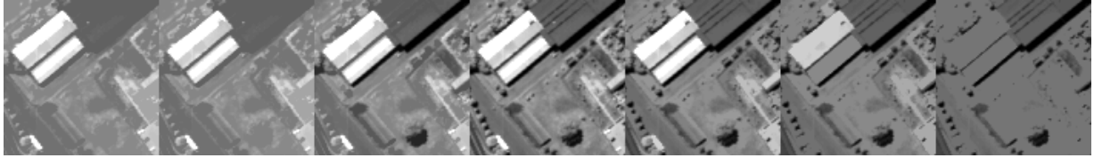
Figure 2.2.: Morphological profile constructed with three opening/closing by reconstruction with a circular SE of size 2, 6 and 10. The left part corresponds to the closings by reconstruction and the dark objects are progressively deleted, e.g., the shadow of the big tree in the middle of the image. The right part corresponds to the openings by reconstruction and the bright objects are progressively deleted, e.g. the buildings in the upper part of the image.
