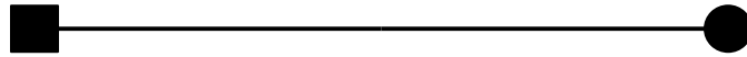
Figure 4.2: Single leaky pipe used to simulate inertia phenomena, connecting a tank ■ to a junction ●.
