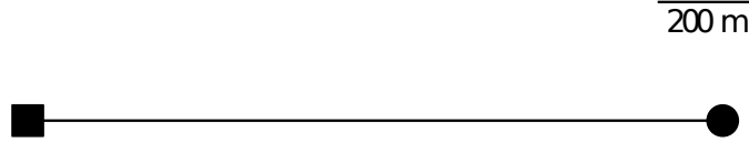
Figure 2.2: Single leaky pipe of length \ell = 1,500 m, connecting a tank ■ to a junction ●.
