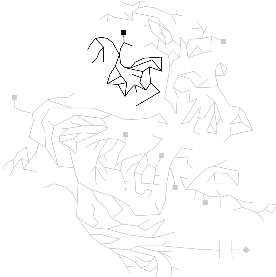
Figure 4.4: In black: district metered area (DMA) of the adapted network C-Town, used to simulate inertia phenomena. In gray: other DMAs (not used). The \blacksquare/\blacksquare represent the tanks. The \blacklozenge represents a reservoir.
