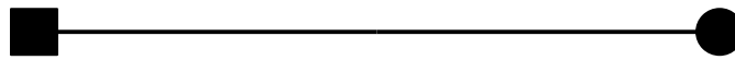
Figure 4.2: Single leaky pipe used to simulate inertia phenomena, connecting a tank ■ to a junction ●.
