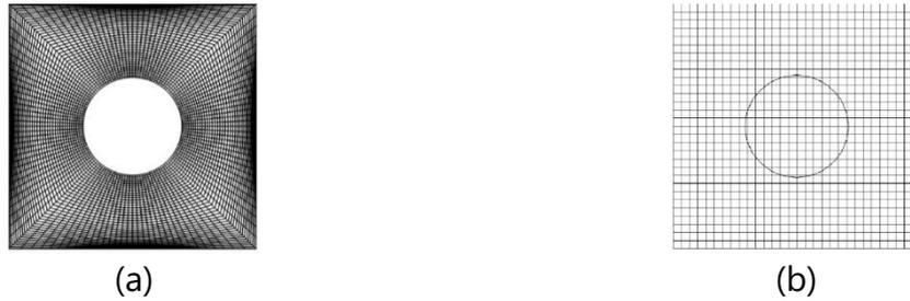
**Figure 1.9** Comparison between (a) conventional mesh and (b) mesh for IBM for a 2D cavity with a circular cylinder (Bansal, 2015)
