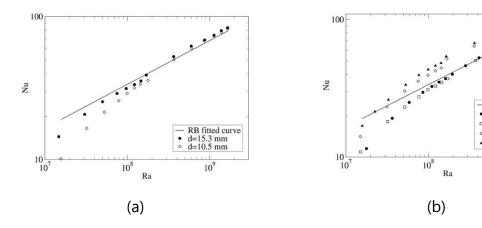
**Figure 1.15** Effect of (a) size of glass sphere and (b) sphere's material at d = 15.3 mm on average Nusselt number in a cavity - RB fitted curve represents the case when Rayleigh-Bénard (RB) convection takes place in the cavity (Ataei-Dadavi et al., 2019)
