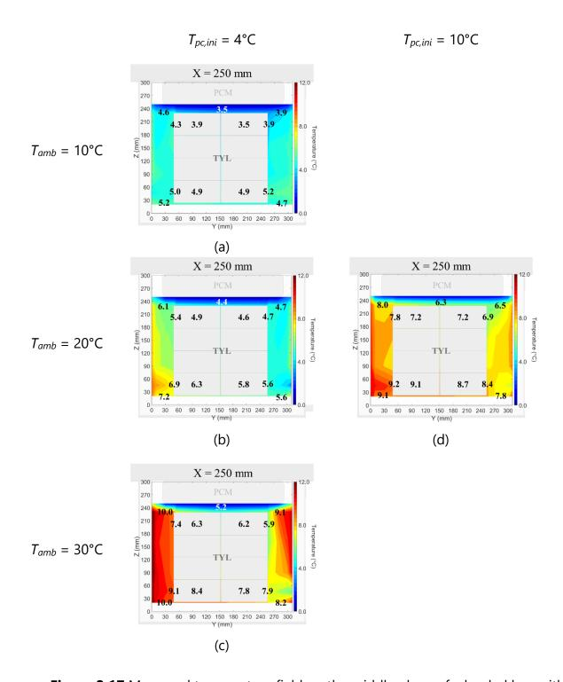
**Figure 2.17** Measured temperature field on the middle plane of a loaded box with PCM at the top and a product initial temperature of 4°C under (a) 10°C ambient temperature – condition 5; (b) 20°C ambient temperature – condition 2; (c) 30°C ambient temperature – condition 6; and (d) product initial temperature of 10°C – condition 8 under 20°C ambient temperature
