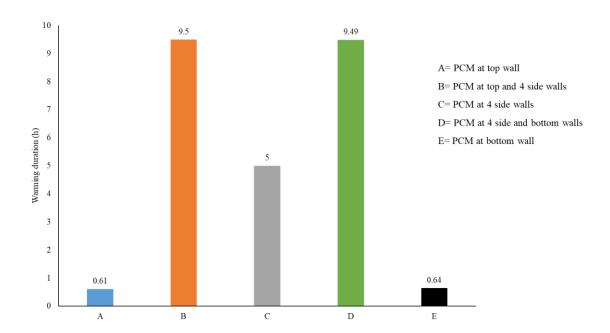
**Figure 1.2** Influence of PCM position and surface area in an insulated box on warming duration defined as the duration during which the temperature at the center of the box rises from 0 °C to 8 °C. Adapted from Du et al. (2020) for a polyurethane box with PCM of 5°C melting point.
