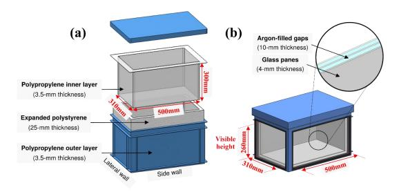
**Figure 2.1** Insulated boxes: (a) commercially manufactured box for temperature measurement (Box A); and (b) box with two walls replaced with triple-glazed windows for velocity measurement (Box B).
