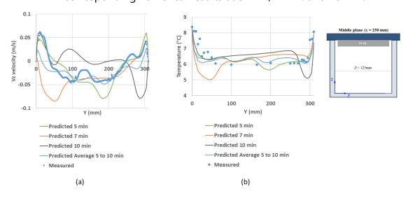
**Figure 3.13** Comparison between experimental and numerical results at t = 5 min., 7 min., 10 min. and average between 5 min. and 10 min. in an unloaded box with PCM at the top at the middle plane and z = 125 mm of (a) air velocity in the z-direction and (b) air temperature
