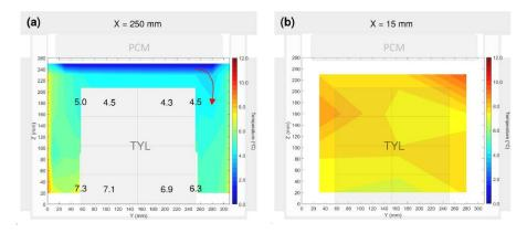
**Figure 2.14** Air temperature field on (a) the middle (x = 250 mm) and (b) the lateral (x = 15 mm) planes of the box with PCM on the lid. Values indicate the timeaveraged core and surface temperatures of the test packs.
