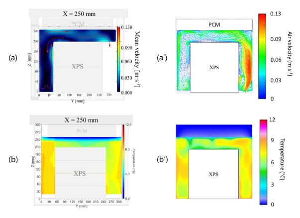
**Figure 3.19** (a) Experimental air velocity field and (b) experimental temperature field on the middle plane of a box with PCM at the top loaded with XPS. (a') and (b') are corresponding numerical results
