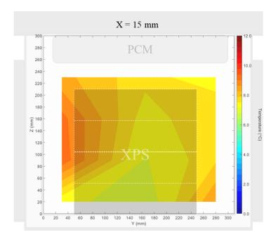
Figure 14: Temperature field at X = 15 mm in a box loaded with XPS and PCM at top
