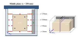
**Figure 2.15** Experimental setup and thermocouple positions in the horizontal box with PCM on a side wall and loaded with the test product (Tylose, TYL). Note: Similar setup and measured positions were applied for the vertical box.
