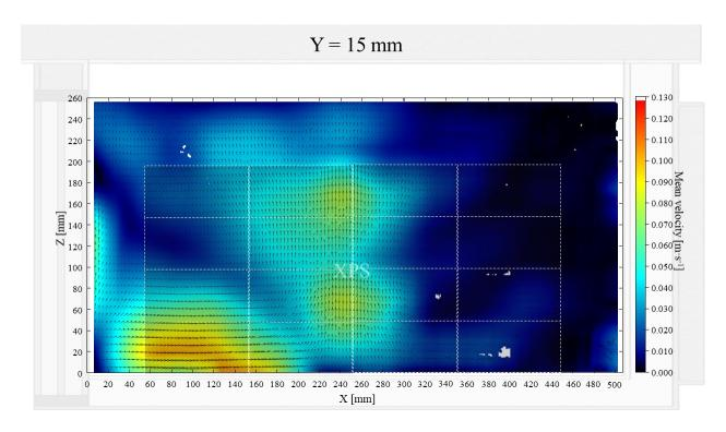
Figure 8: Air velocity field at Y = 15 mm in a box loaded with XPS and PCM on a side
