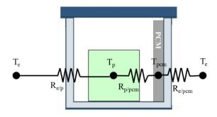
Figure 4.1 Lumped model structure
