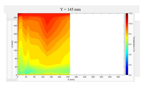
Figure 3: Temperature field at Y = 145 mm in an unloaded horizontal box with PCM on a side
