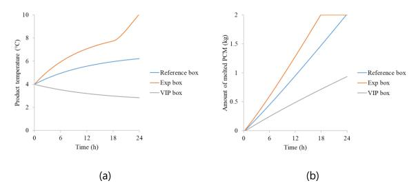
**Figure 4.10** Effect of box insulation on: (a) average product temperature evolution; and (b) the amount of melted PCM estimated by the lumped model. The initial product and PCM temperatures were 4°C and -2°C, respectively
