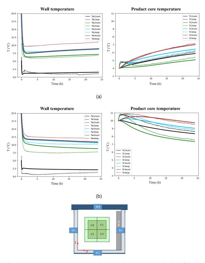
**Figure 3.6** Comparison between numerical results and the experimental values of the temperature evolution during 24 h at the level of the wall and the product core in an insulated box equipped with PCM on one side during transient state with an ambient temperature of 20°C and an initial test product temperature of (a) 4°C (reference condition) and (b) 10°C
