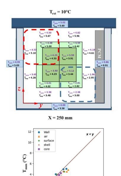
**Figure 3.4** Comparison between the numerical and experimental values of temperature at steady state in an insulated box equipped with PCM on one side with an ambient temperature of (a) 20°C (reference condition) and (b) 10°C. The zones with the lowest and highest temperatures are surrounded in blue and red lines, respectively.
