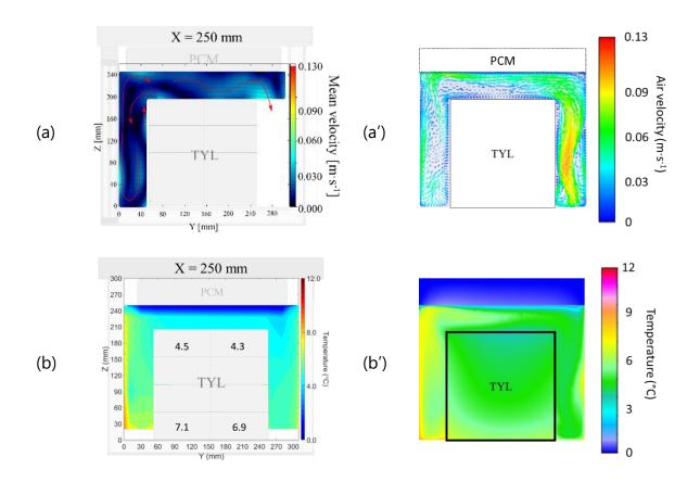
**Figure 3.20** (a) Experimental air velocity field and (b) experimental temperature field on the middle plane of a box with PCM at the top loaded with Tylose. (a') and (b') are corresponding numerical results with initial air and Tylose temperature of 20°C and 4.3°C, respectively.
