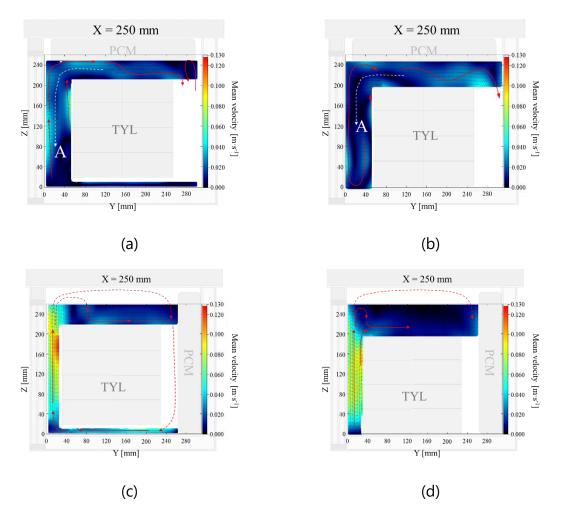
**Figure 2.18** Measured air velocity field on the middle plane of a loaded box (a) PCM at the top, 20-mm gap underneath the test product – condition 2, (b) PCM at the top, without gap – condition 10, (c) PCM on the side, 20-mm gap underneath the test product – condition 1 and (d) PCM on the side, without gap – condition 9
