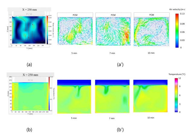
**Figure 3.12** (a) Experimental air velocity field and (b) experimental temperature field on the middle plane of an unloaded box with PCM at the top. (a') and (b') are corresponding numerical results at 5 min., 7 min. and 10 min.
