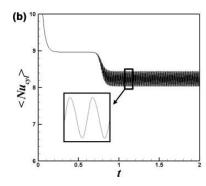
**Figure 1.12** Time history (using dimensionless time value) versus surface-averaged Nusselt number of a heated cylinder in a cavity with heated bottom wall and top cold wall at (a)  $Ra = 10^4$  and (b)  $Ra = 10^6$  (Lee et al., 2013)
