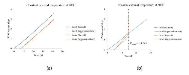
**Figure 4.9** Required PCM amount (orange curves) as a function of the maximum storage period (t<sub>max</sub>) for a maximum product temperature of 8°C by direct calculation and approximation under (a) constant 20°C ambient temperature, and (b) constant 30°C ambient temperature. The product and PCM initial temperatures were 4°C and - 2°C, respectively. The blue curves also indicate the melting period (t<sub>melt</sub>).
