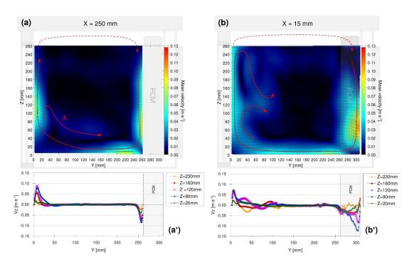
**Figure 2.5** Air velocity fields on (a) the middle (x = 250 mm) and (b) the lateral (x = 15 mm) planes of the box with PCM on the side wall. (a') and (b') are the profiles of the vertical velocity component ( $v_z$ ) at 4 heights on the middle and the lateral planes, respectively.
