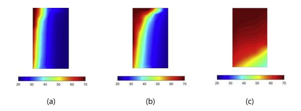
**Figure 1.16** Temperature field in a melting PCM (paraffin waxes  $-T_m = 55.0$ °C) at (a) 40 min, (b) 80 min and (c) 600 min (Jevnikar & Siddiqui, 2019)
