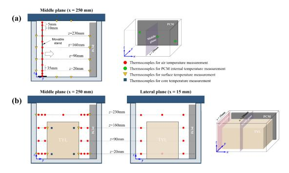
**Figure 2.2** Diagram showing the experimental setup for temperature measurement for PCM located on the side wall of (a) empty box, and (b) loaded box. TYL = Tylose packages.
