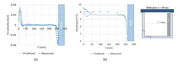
**Figure 3.11** Comparison between experimental and numerical results at the middle plane and z = 160 mm in an unloaded box with PCM on a sidewall (a) air velocity in the z-direction and (b) air temperature
