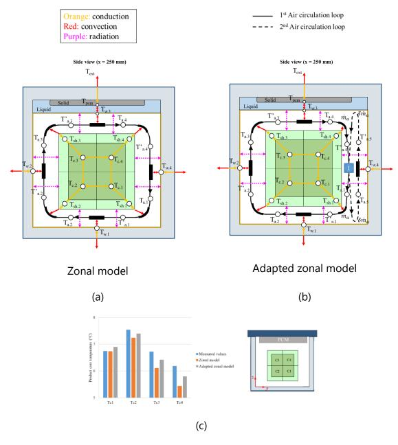
**Figure 4.14** Heat transfer and airflow diagram in a 2D insulated box with PCM at the top for (a) the zonal model; (b) the adapted zonal model; and (c) comparison between the average core temperature at 4 measured positions and numerical values under steady state using an experimental box
