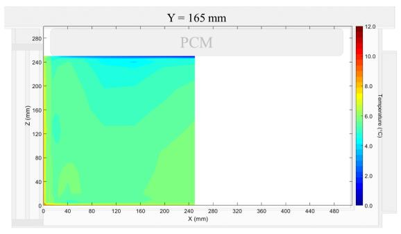
Figure 6: Temperature field at Y = 165 mm in an unloaded horizontal box with PCM at top
