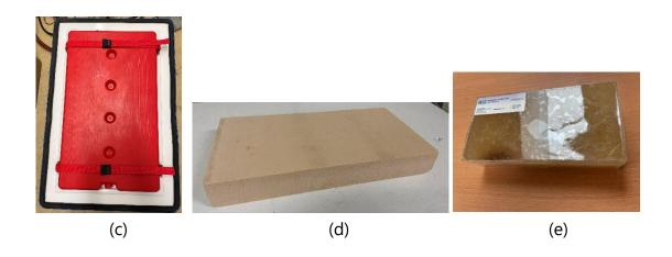
Figure 15: Materials and experimental setup (a) the box with wood support on the table, (b) experimental setup, (c) PCM container, (d) extruded polystyrene slab, and (e) test product pack
