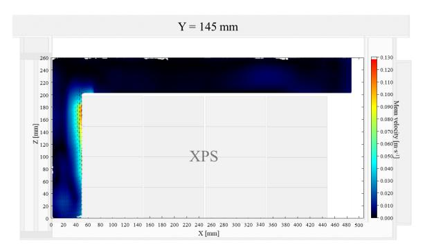
Figure 7: Air velocity field at Y = 145 mm in a box loaded with XPS and PCM on a side. White area on the right represents the unmeasurable zone because of the inaccessibility of laser sheet.
