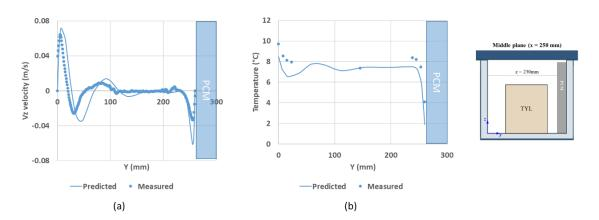
**Figure 3.17** Comparison between experimental and numerical results in a box loaded with Tylose with PCM on a sidewall at the middle plane and z = 230 mm of (a) air velocity in the z-direction and (b) air temperature
