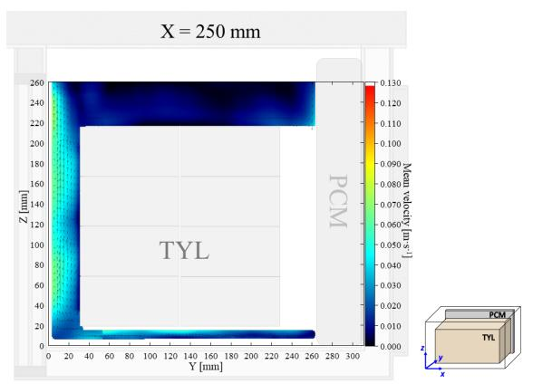
Figure 4: Air velocity field at X = 250 mm in a loaded horizontal box with PCM on a sidewall under 30°C ambient, product initial temperature = 4°C with 20 mm gap below. White area on the right represents the unmeasurable zone because of the inaccessibility of laser sheet.
