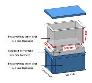
**Figure 4.2** Insulated box used in the experimental validation (Source: Leungtongkum et al. (2023a)).
