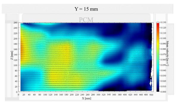
Figure 5: Air velocity field at Y = 15 mm in an unloaded horizontal box with PCM at top
