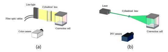
**Figure 1.8** Experimental setup for (a) temperature field measurement by LCT and (b) velocity field measurement by PIV (Ataei-Dadavi et al., 2019)
