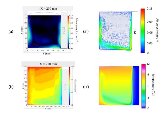
**Figure 3.10** (a) Experimental air velocity field and (b) experimental temperature field on the middle plane of an unloaded box with PCM on a sidewall. (a') Corresponding numerical air velocity field and (b') Corresponding numerical temperature field.
