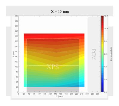
Figure 10: Temperature field at X = 15 mm in a box loaded with XPS and PCM on a side
