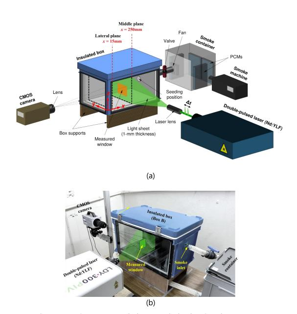
Figure 2.3 Diagram (a) and photograph (b) showing the PIV setup.
