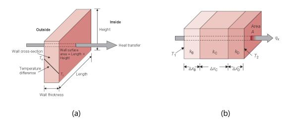
**Figure 1.4** Heat conduction through (a) a single slab and (b) a series of rectangular slabs (Singh et al., 2008a)
