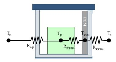
Figure 3.1 Lumped model structure
