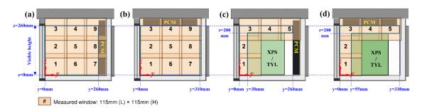
**Figure 2.4** Position of measured windows for the PIV measurement: (a) empty box/PCM on the side wall, (b) empty box/PCM on the lid, (c) loaded box/PCM on the side wall, and (d) loaded box/PCM on the lid.
