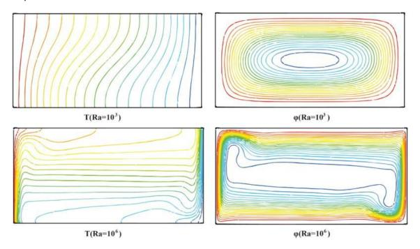
**Figure 1.11** Isotherms (left) and streamlines (right) of an empty cavity with vertical warm and cold wall and adiabatic horizontal walls (Rincón-Casado et al., 2017)
