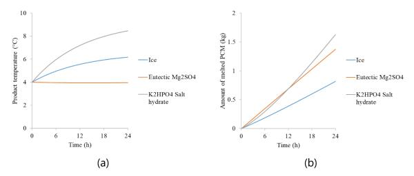
**Figure 4.11** Effect of the PCM type on: (a) product temperature evolution; and (b) PCM melted mass evolution calculated by the lumped model; the product initial temperature was 4°C
