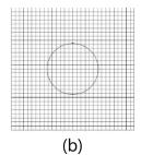
**Figure 1.9** Comparison between (a) conventional mesh and (b) mesh for IBM for a 2D cavity with a circular cylinder (Bansal, 2015)
