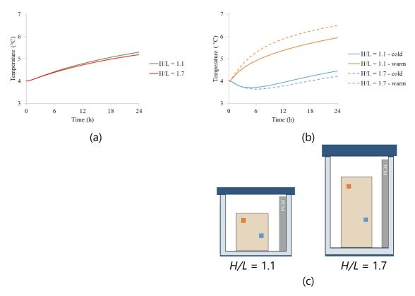
**Figure 4.17** The effect of the aspect ratio (*H/L*) of the box on: (a) average load temperature evolution; and (b) load temperature evolution at the coldest and warmest points; (c) position of the coldest (■) and warmest (■) points.
