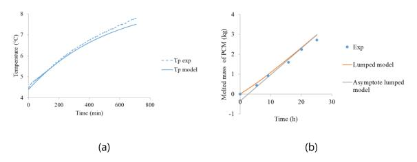
**Figure 4.3** Comparison between the experimental and numerical values (by lumped model) in a box with PCM on a side wall under 20°C ambient: (a) product temperature evolution with  $T_{p,0} = 4.4$ °C, and (b) melted PCM mass
