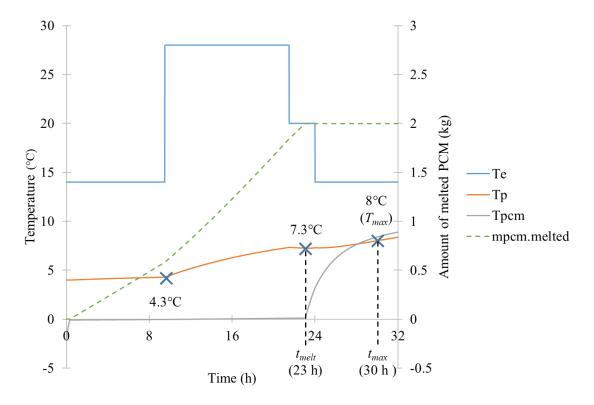
**Figure 4.8** Product  $(T_p)$  and PCM  $(T_{pcm})$  temperatures, melted PCM mass evolution  $(m_{pcm.melted})$  under varying ambient conditions  $(T_e)$  predicted by the lumped model; the product and PCM initial temperatures were 4°C and -2°C, respectively, PCM mass 2 kg.
