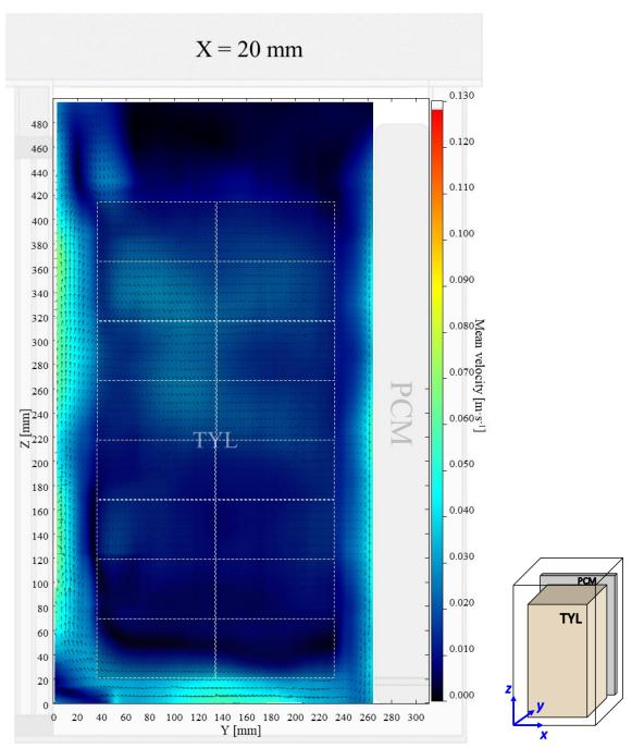
Figure 3: Air velocity field at X = 20 mm in a loaded vertical box with PCM on a sidewall under 20°C ambient, product initial temperature = 4°C with 20 mm gap below
