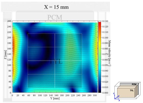
Figure 2: Air velocity field at X = 15 mm in a loaded horizontal box with PCM at the top under 20°C ambient, product initial temperature = 4°C with 20 mm gap below
