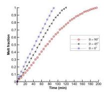
**Figure 1.18** Effect of inclination angle of a PCM cavity on melt fraction evolution –  $\theta$  = 0° is horizontally PCM and  $\theta$  = 90° is vertically PCM (Kamkari et al., 2014)
