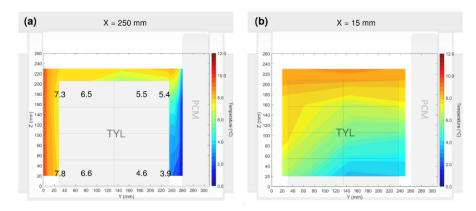
**Figure 2.12** Air temperature field on (a) the middle (x = 250 mm) and (b) the lateral (x = 15 mm) planes of the box with PCM on the side wall. Values indicate the time-averaged core and surface temperatures of the test products.
