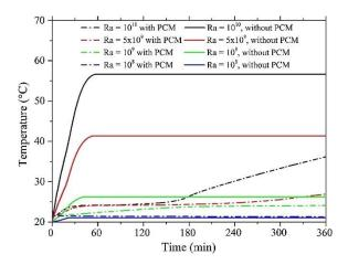
Figure 1.19 Temperature evolution in a cavity without and with PCM (PureTemp29X  $-T_m = 28.6 - 29.4$ °C) at various Rayleigh number (Moreno et al., 2020)
