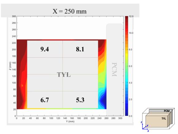
Figure 5: Air temperature field and core temperature of test product (°C) at X = 250 mm in a loaded horizontal box with PCM on a sidewall under 30°C ambient, product initial temperature = 4°C with 20 mm gap below
