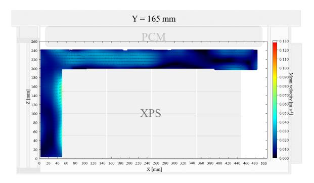
Figure 11: Air velocity field at Y = 165 mm in a box loaded with XPS and PCM at top.
