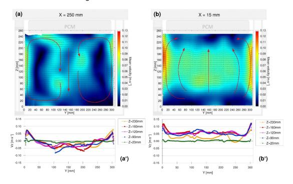
**Figure 2.7** Air velocity fields at (a) the middle (x = 250 mm) and (b) the lateral (x = 15 mm) planes of the box equipped with PCM on the lid. The profiles of the z-component of the velocity at 4 heights on (a') the middle and (b') the lateral planes.
