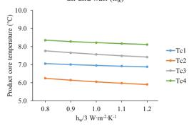
Convective heat transfer coefficient between internal air and product surface  $(h_p)$
