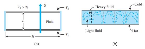
**Figure 1.6** (a) A horizontal enclosure with isothermal surfaces and adiabatic vertical walls and (b) fluid flow pattern inside an enclosure (Cengel & Ghajar, 2020)
