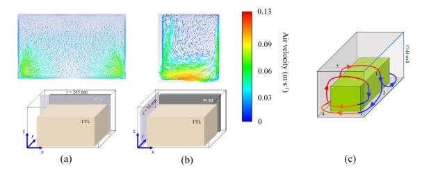
**Figure 4.16** CFD results of air velocity field at t = 24 h (a) near an PCM surface, y = 245 mm (b) near lateral wall, x = 15 mm, and (c) 3D airflow illustration (in a loaded box with PCM on a side wall)
