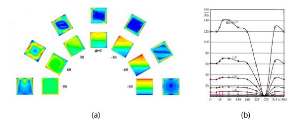
**Figure 1.13** Effect of inclination angle of a cavity on (a) velocity map (on the outer radius) and temperature map (on the inner radius) and (b) average Nusselt number versus inclination angle for various Rayleigh number (Baïri, 2008)
