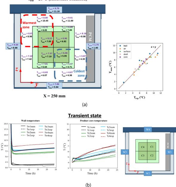
**Figure 4.5** Comparison between the experimental and numerical (by zonal model) temperatures in an insulated box equipped with PCM on one side wall with an initial product temperature of 4°C and ambient temperature of 20°C: (a) steady state, and (b) transient state. Source: Leungtongkum et al. (2023b)
