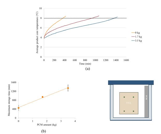
**Figure 2.20** Effect of the amount of PCM on (a) test product core temperature evolution; and (b) maximum storage time, t<sub>max</sub>. Error bars represent the standard deviation of 2 replications. The experiment was conducted under condition 4: loaded box with PCM on a sidewall with an ambient temperature of 20°C, 4°C initial product temperature, 20 mm gap beneath the test product (Tylose, TYL)
