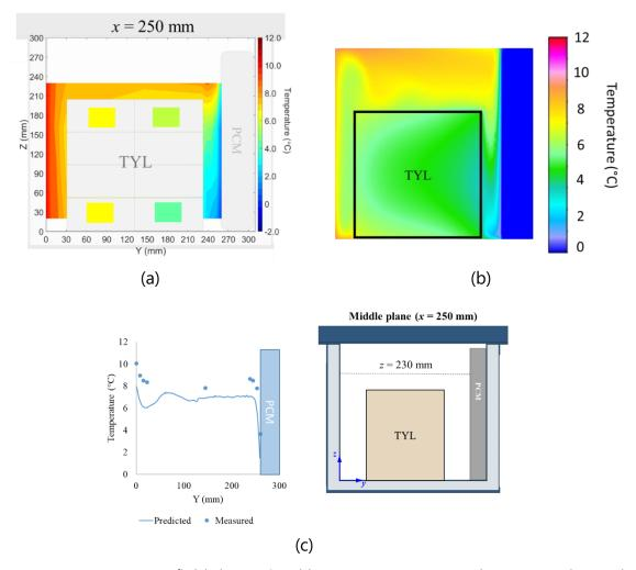
**Figure 4.6** Temperature field determined by: (a) measurement, (b) CFD results, and (c) comparison between experimental and CFD results at t = 4 h of air temperature at z = 230 mm on the middle plane. Box loaded with test product (Tylose, TYL) with PCM on a side wall.
