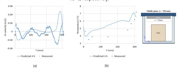
**Figure 3.21** Comparison between experimental and numerical results in a box loaded with Tylose with PCM at the top at the middle plane and z = 230 mm of (a) air velocity in z-direction and (b) air temperature
