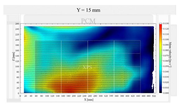
Figure 12: Air velocity field at Y = 15 mm in a box loaded with XPS and PCM at top
