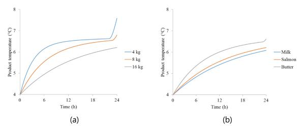
**Figure 4.12** Effect of: (a) a mass of salmon, and (b) the nature of the product (16 kg of salmon, butter or milk) on the product temperature evolution calculated by lumped model for a PCM mass of 2 kg. The product and PCM initial temperatures were 4°C and -2°C, respectively.
