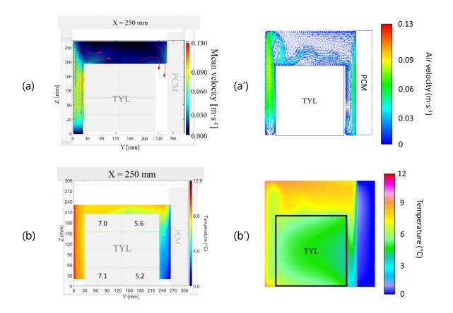
**Figure 3.15** (a) Experimental air velocity field and (b) experimental temperature field on the middle plane of a box loaded with Tylose with PCM on a sidewall. (a') and (b') are corresponding numerical results with initial air and Tylose temperature of 20°C and 4.4°C, respectively
