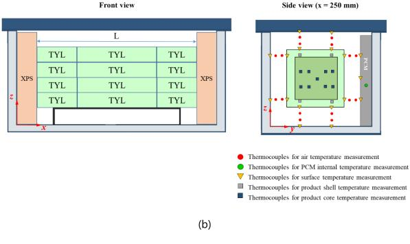
**Figure 3.3** (a) Insulated box; and (b) experimental set-up of a box loaded with the test product (Tylose, TYL) and 50-mm extruded polystyrene plates (XPS) on the lateral walls to prevent airflow, and thermocouple positions
