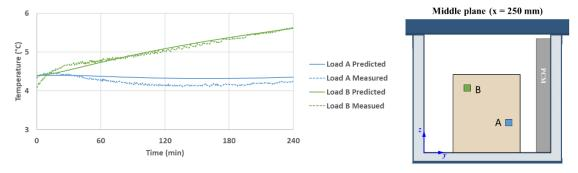
**Figure 3.18** Comparison between experimental and numerical results of temperature evolution at two positions in Tylose slab in a box loaded with Tylose with PCM on a sidewall from the beginning to 4 h
