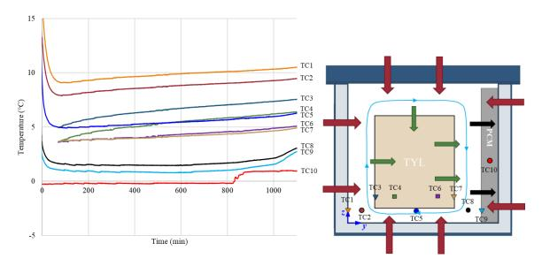
**Figure 2.19** Temperature evolution at the bottom of the box during experiment No. 1 (ambient temperature = 20°C and initial test product temperature = 4°C) with heat flow (red arrows – from ambient, green arrows – between the internal air and the test product, and black arrows – from the internal air to the PCM). Airflow shown using blue arrows
