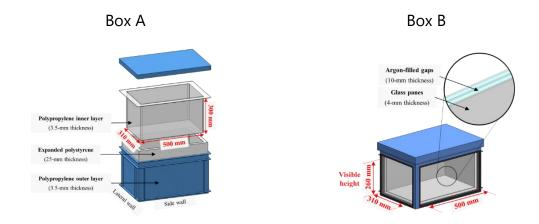
**Figure 3.7** Boxes used in the study. Box A: a commercial box for temperature measurement and Box B: a box with walls modification by triple-pane windows for velocity measurement.
