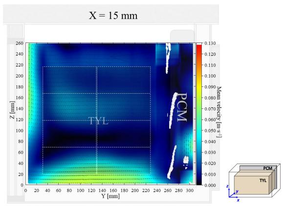
Figure 1: Air velocity field at X = 15 mm in a loaded horizontal box with PCM on a sidewall under 20°C ambient, product initial temperature = 4°C with 20 mm gap below. Note: unmeasured air velocity in white areas on the right can be explained by the refraction from PCM surface behind the laser sheet.
