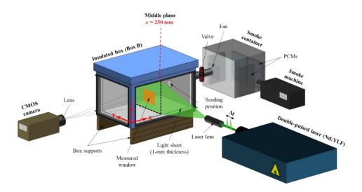
**Figure 3.9** Diagram showing the PIV setup.
