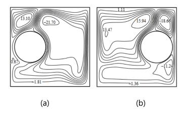
**Figure 1.14** Effect of position of a heated circular cylinder on streamlines in a cavity (hot wall on the left and cold wall on the right) at  $Ra = 10^6$  with (a) cylinder on the left and (b) cylinder on the right (Jami et al. 2008)
