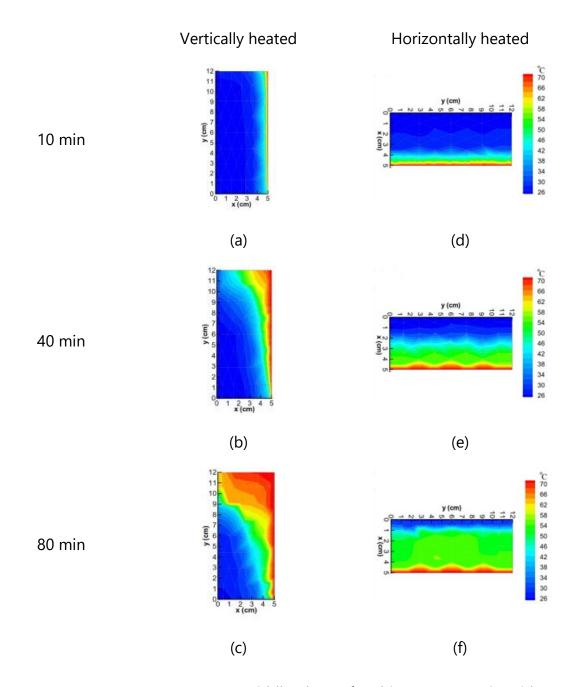
**Figure 1.17** Temperature contour at middle plane of melting PCM (Lauric acid  $-T_m = 43.5$  to 48.2°C) (a - c) vertically heated (d - f) horizontally heated at 10, 40 and 80 min. (Kamkari et al., 2014)
