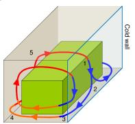
**Figure 2.11** Illustration of three-dimentional flow in a box with PCM on the side wall. Numbers indicate the states of the flow.
