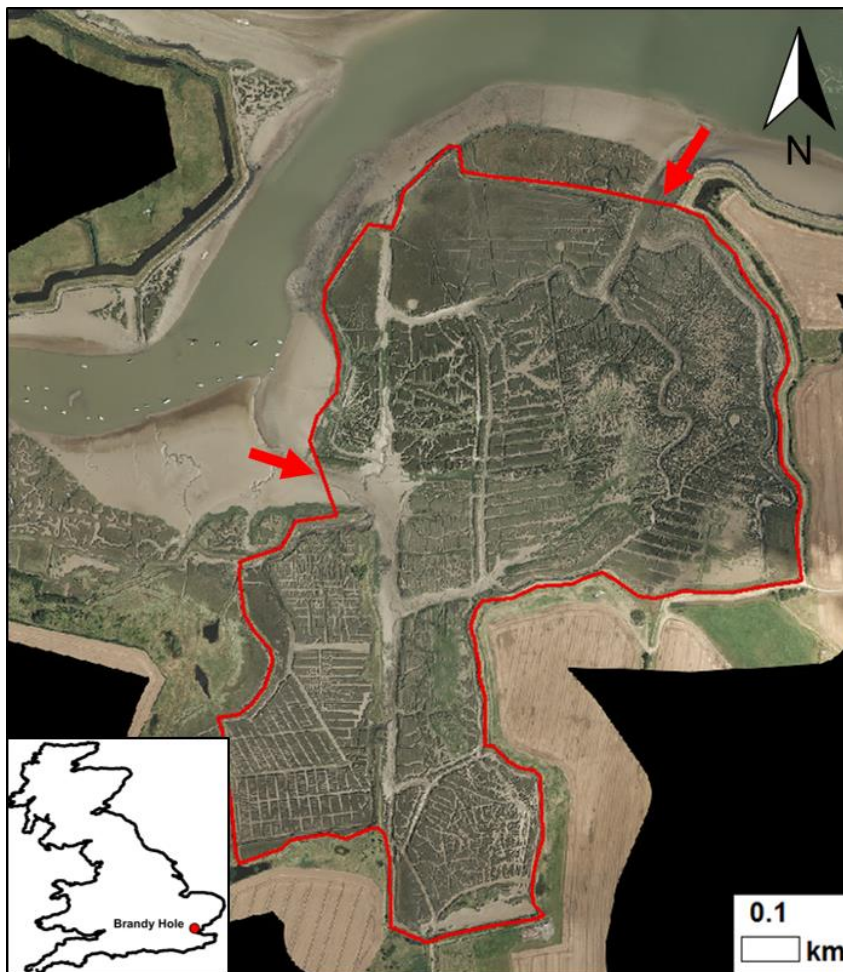
Figure 3.29: Aerial photograph of Brandy Hole (20 cm resolution composite image from two flights on the 06/05/2016 and 23/09/2016, Environment Agency). Breaches shown by red arrows. AR extent considered shown by red line.
