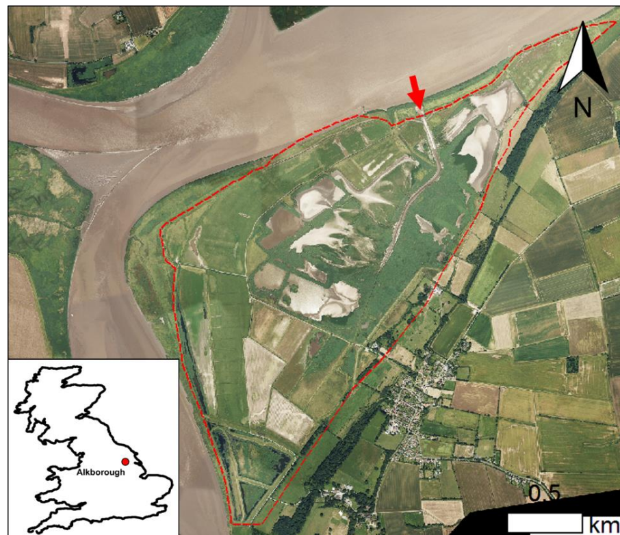
Figure 3.23: Aerial photograph of Alkborough (20 cm resolution composite image from two flights on the 07/05/2016 and the 23/08/2016, Environment Agency). Breach area shown by red arrow. MR extent considered shown by dashed red line.
