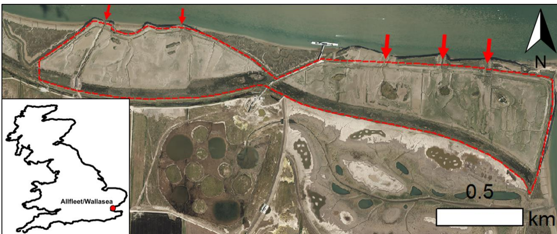
Figure 3.24: Aerial photograph of Allfleet/Wallasea (20 cm resolution composite image from two flights on the 06/05/2016 and the 23/09/2016, Environment Agency). Breaches shown by red arrows. MR extent considered shown by dashed red line.
