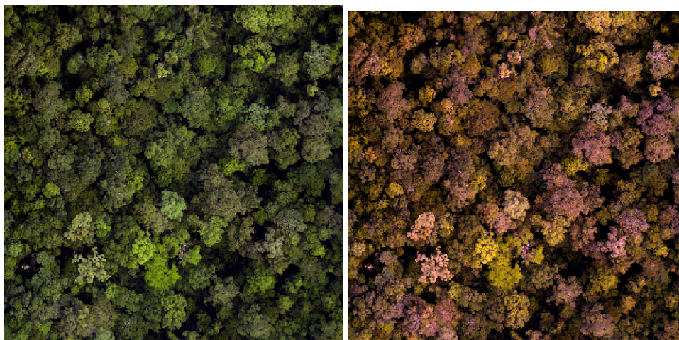
Fig. B.1 An original RGB image is displayed on the left, while a contrasted enhanced (stretched) RGB image is displayed on the right of this figure. Stretching the colours of the image to the values allows for easier identification of individual trees when carrying out manual tree crown delineations. The effect is particularly noticeable in the lower left corner of the images.
