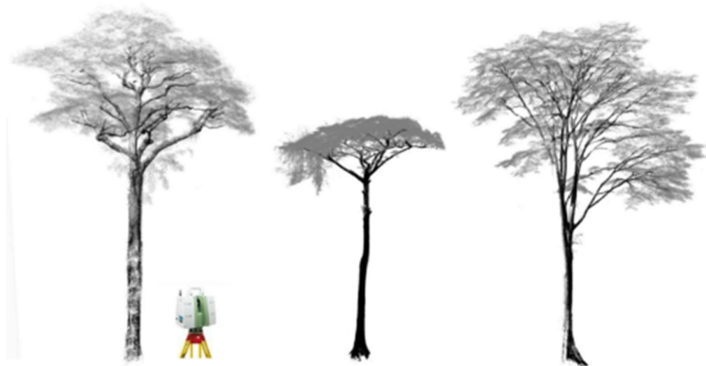
Figure 36. Trees scanned with terrestrial LiDAR. From left to right, Triplochytton scleroxylon , Terminalia superba , Piptadeniastrum africanum .
